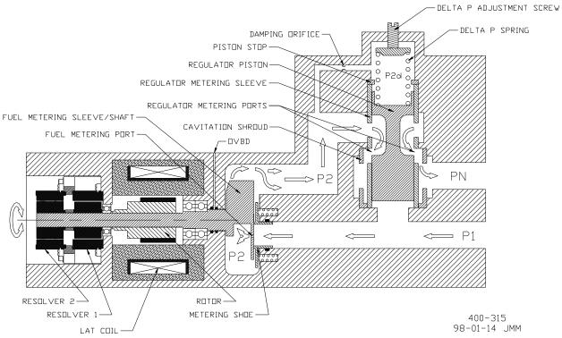
Figure 1-1. LQ6T Valve Schematic
