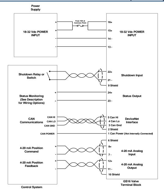
Figure 2-6. LQ6T / LQ6BP Plant Wiring Diagram
