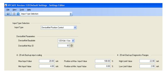
Figure 4-22. DeviceNet Position Control
