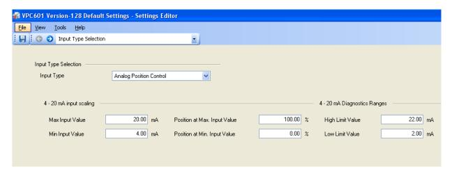
Figure 4-19. Analog Position Control
