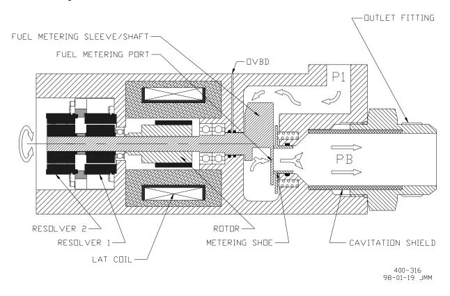
Figure 1-2. LQ6BP Valve Schematic
