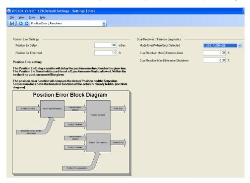
Figure 4-26. Position Error/Resolver Setting Screen
