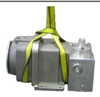
Figure 2-2. Using a Sling to Lift the Valve
