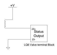
The two methods for wiring the Status Output are shown above. The Status Output indicates if the LQ6 is shut down or running. There are two ways for the LQ6 to be shut down—if the Shutdown/Reset input is in shutdown, or if a diagnostic has been triggered. If the LQ6 is in a shutdown situation, the status output is open (no current).
