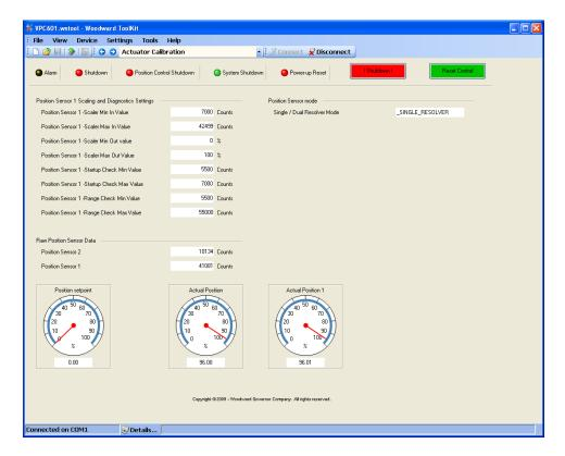
Figure 4-11. Single Resolver Screen
