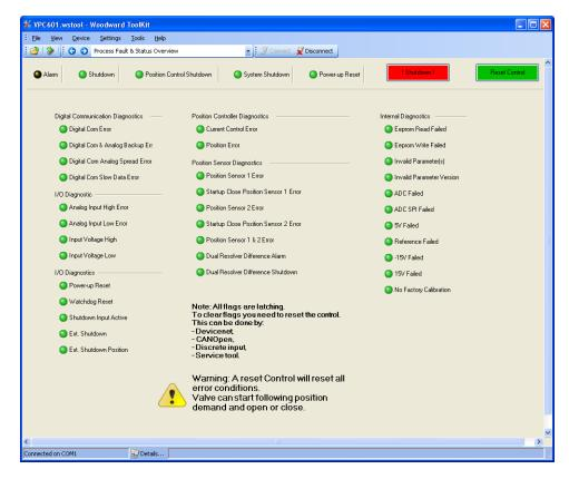
Figure 4-4. Process Fault & Status Overview
