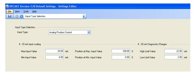
Figure 4-28. Analog Position Control
