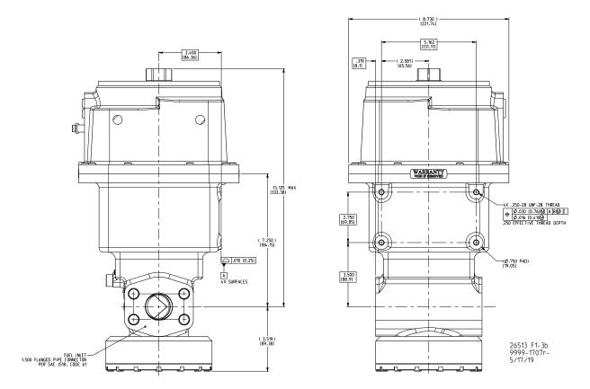
Figure 1-3b GS6FS Outline Drawing (Measurements Shown in Inches)
