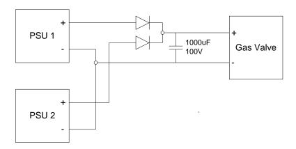
Figure 2-5. Recommended Parallel Power Supply Connection
