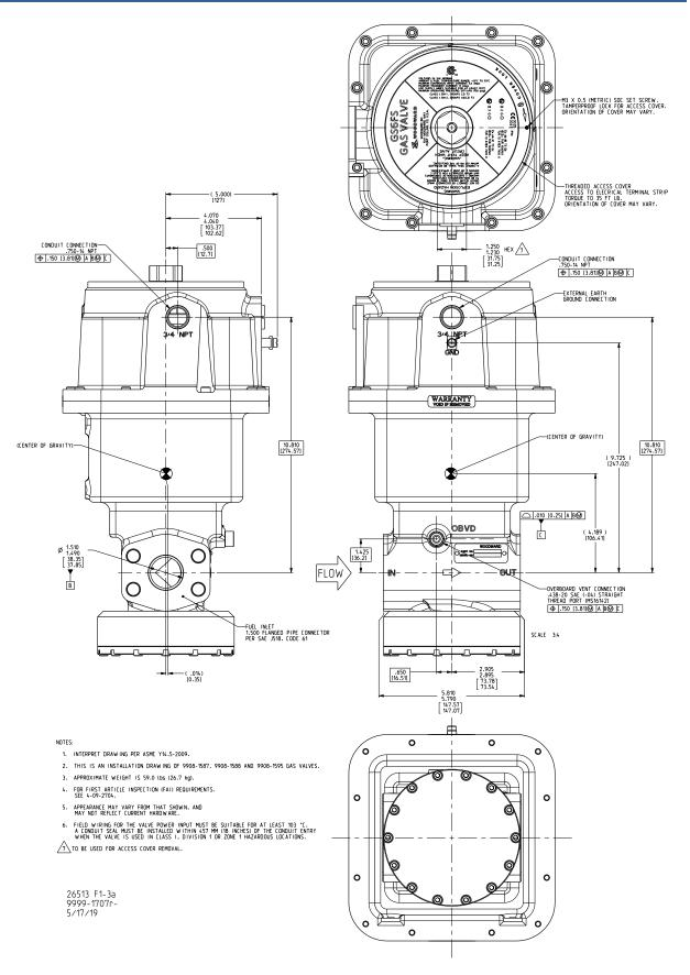
Figure 1-3a. GS6FS Outline Drawing (Measurements Shown in Inches)
