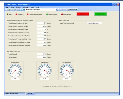
Figure 4-20. Single Resolver Screen
