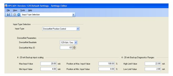
Figure 4-31. DeviceNet Position Control
