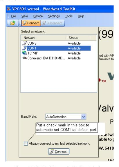
Figure 4-4. VPC Tool Communication Port Selection
