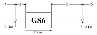
Figure 2-1. Piping Requirements
