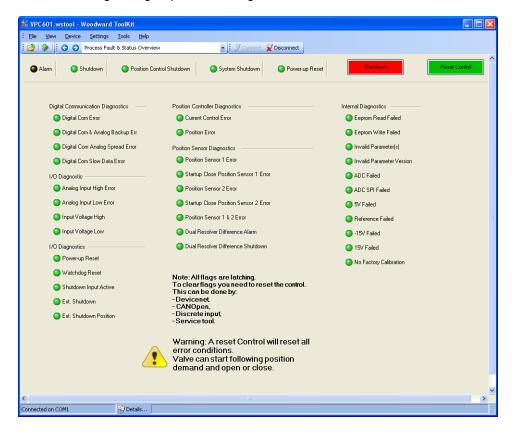
Figure 4-13. Process Fault & Status Overview
