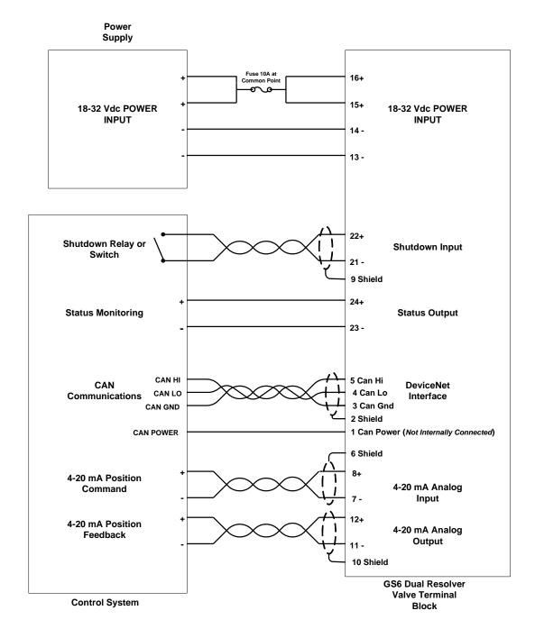
Figure 2-4. GS6 Plant Wiring Diagram
