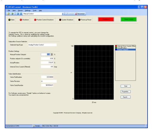
Figure 4-9. Manual Control Screen
