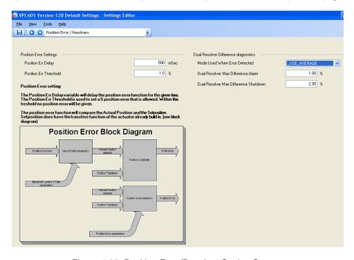
Figure 4-35. Position Error/Resolver Setting Screen
