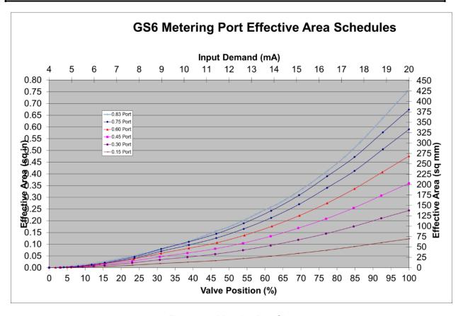
Figure 6-1. Metering Port Size
