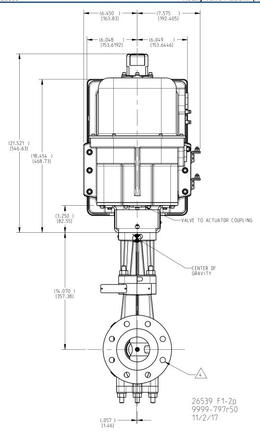
Figure 1-2p. RVP-200 Outline Drawing (90-degree Counter-Clockwise Configuration)
