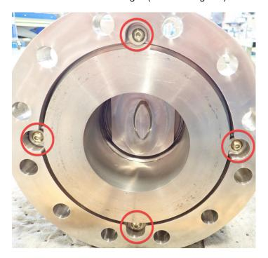
Figure 2-1. Inlet Sleeve Assembly Screws (circled in red)
