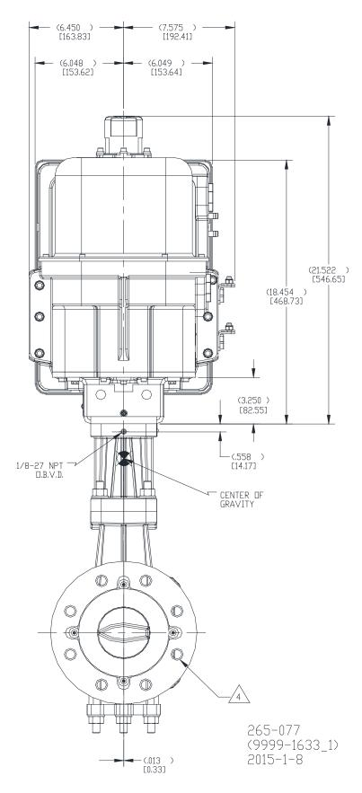
Figure 1-2i. RVP-200 Outline Drawing (90-degree Clockwise Configuration)
