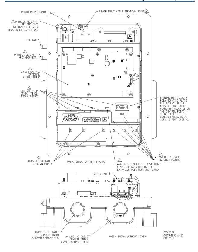
Figure 1-3a. RVP-200 Wiring Diagram
