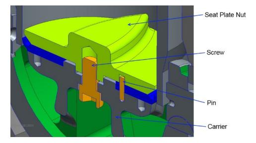
Figure 4-3. Install the Seat Plate and Seat Plate Nut
