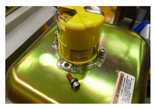
Figure 2-17. Indicator Removal In-Process (IECEx Marked Valve)
