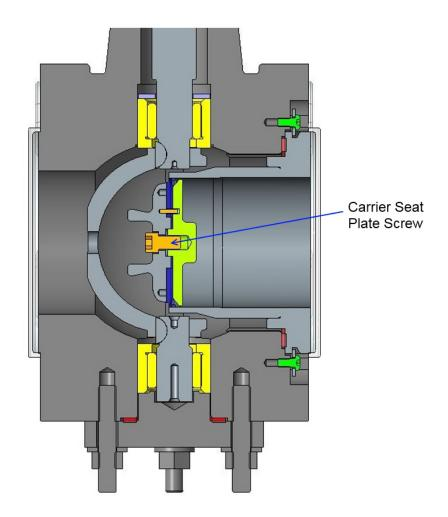
Figure 4-7. Torque the Carrier Seat Plate Screw
