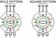
Figure 2-8. Torquing Patterns
