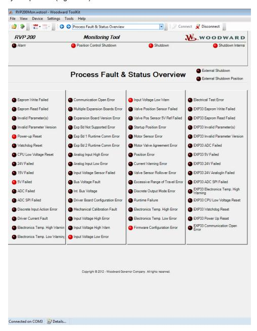
Figure 3-9. Process Fault & Status Overview
