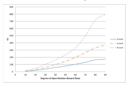
Figure 1-1. RVP Valve Cv Table in Graph Form
