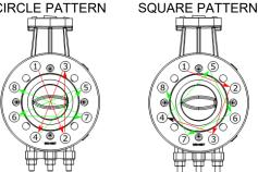
Figure 2-10. Torquing Patterns
