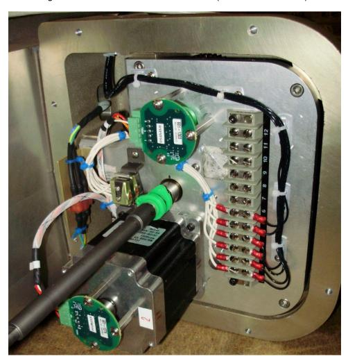
Figure 2-18. Actuator Limit Switch Conduit Entry: Upper Left
