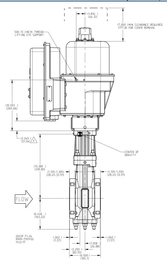
Figure 1-2o. RVP-200 Outline Drawing (90-degree Counter-Clockwise Configuration)
