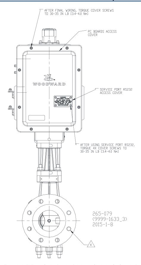
Figure 1-2k. RVP-200 Outline Drawing (90-degree Clockwise Configuration)
