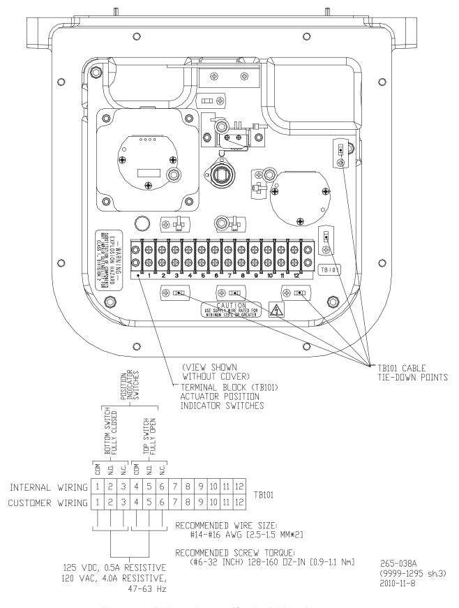
Figure 1-4a. RVP-200 Actuator (Gearbox) Wiring Diagram
