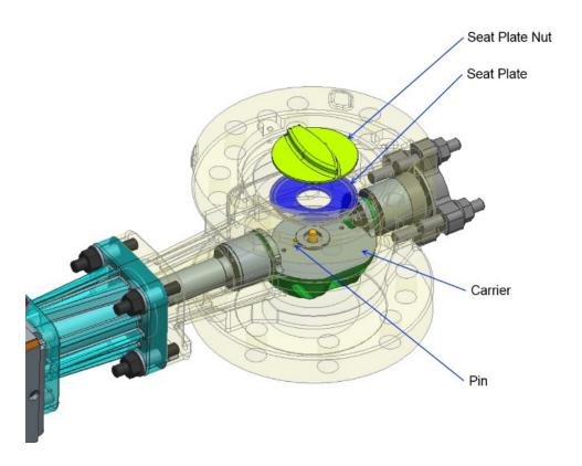
Figure 4-2. Reposition the Valve Assembly, Orient the Seat Plate
