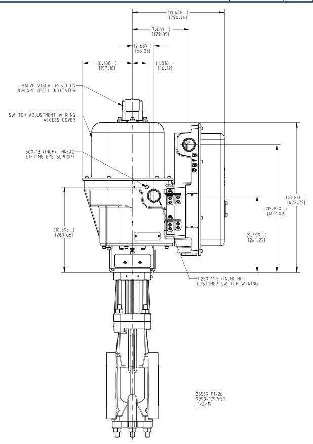
Figure 1-2q. RVP-200 Outline Drawing (90-degree Counter-Clockwise Configuration)
