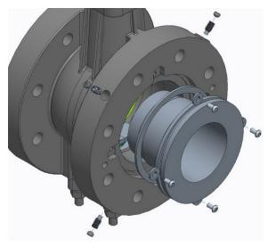
Figure 4-1. Removing the Seat Plate and Sleeve
