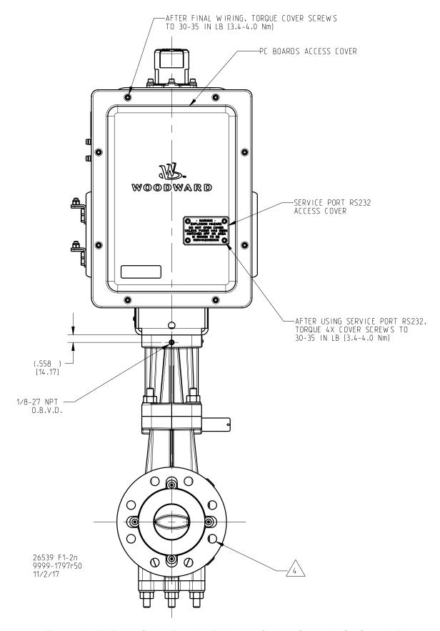
Figure 1-2n. RVP-200 Outline Drawing (90-degree Counter-Clockwise Configuration)
