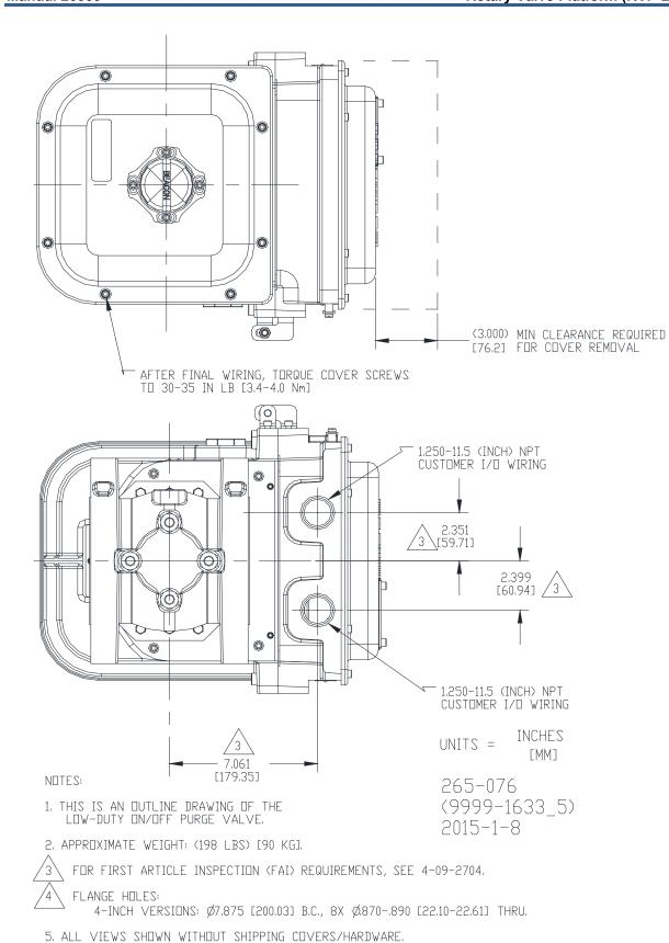
Figure 1-2g. RVP-200 Outline Drawing (90-degree Clockwise Configuration)
