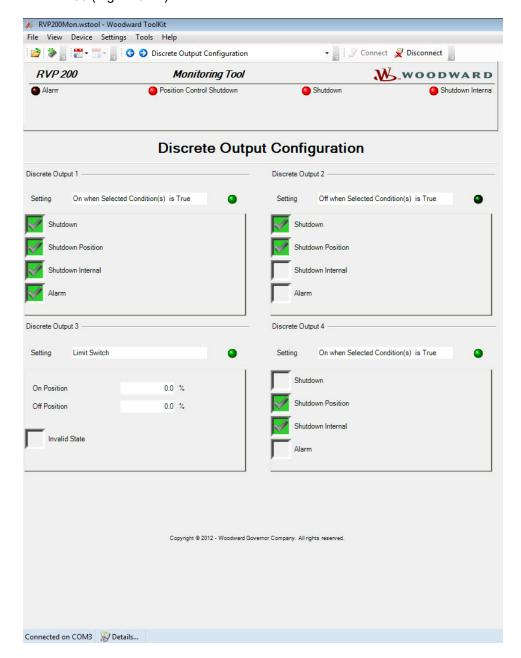
Figure 3-17. Discrete Output Configuration
