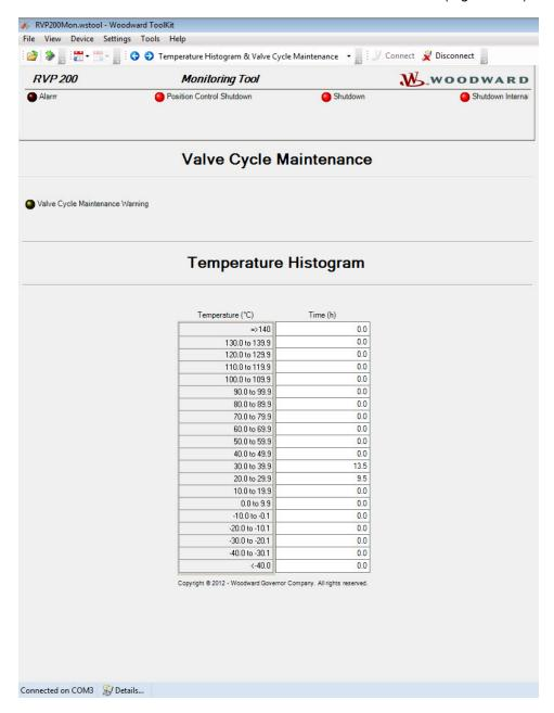
Figure 3-16. Temperature Histogram & Valve Cycle Maintenance
