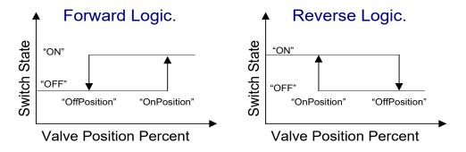
Figure 3-18. Forward and Reverse Logic
