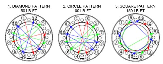
Figure 4-6. Torquing Patterns and Values
