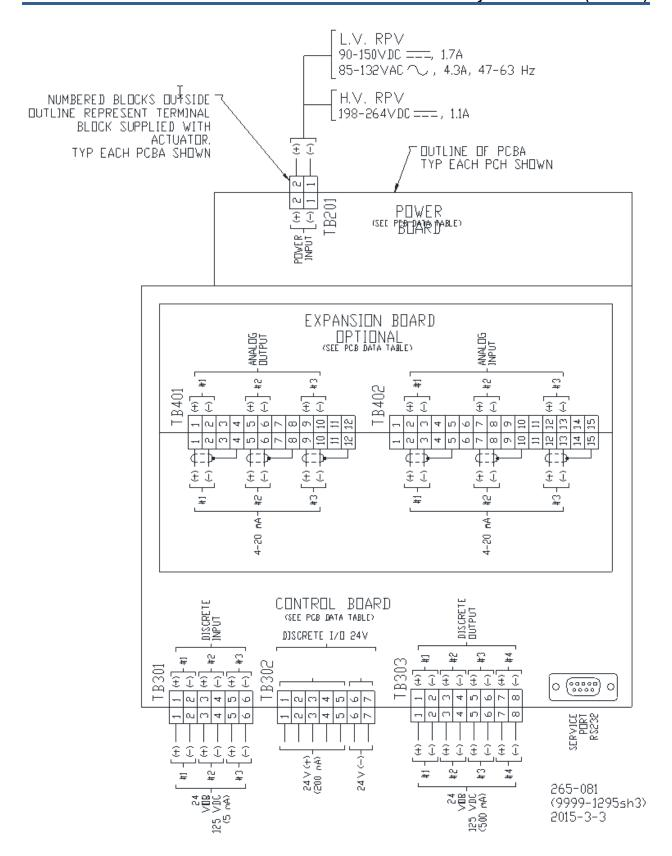
Figure 1-3c. RVP-200 Wiring Diagram
