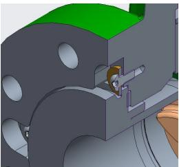
Figure 4-4. Install Spiral Gasket and Sleeve
