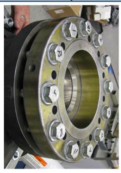
Figure 2-2. Raised Face Inlet Sleeves
