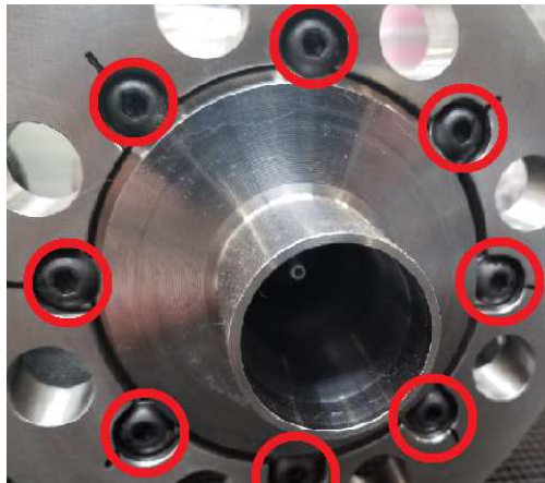
Figure 3-1. Illustration of Diverging Sleeve Screws
