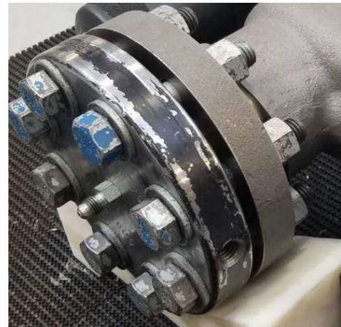
Figure 3-2. Illustration of Raised Face Style Diverging Sleeve
