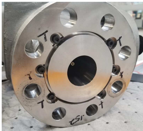
Figure 3-2. Illustration of Raised Face Style Diverging Sleeve
