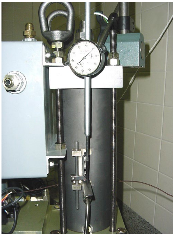
Figure 3-2. Water Valve Piston Rig Tool
