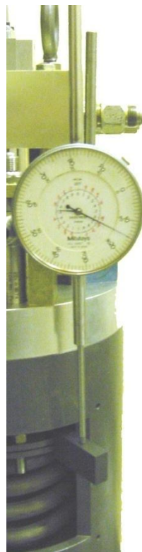
Figure 5-3. Stroke Measurement Attachment Bar
