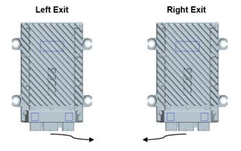
Figure 2-8. SECM Connector Orientations
