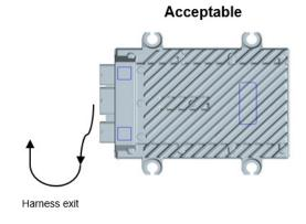
Figure 2-5. Acceptable SECM112 Mounting Orientations
