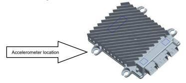
Figure 1-1. Location of Accelerometer to Measure Mounting Vibration
