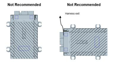
Figure 2-6. Not Recommended SECM112 Mounting Orientations
