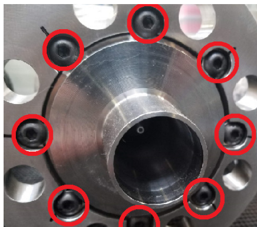
Figure 3-1. Illustration of Diverging Sleeve Screws
