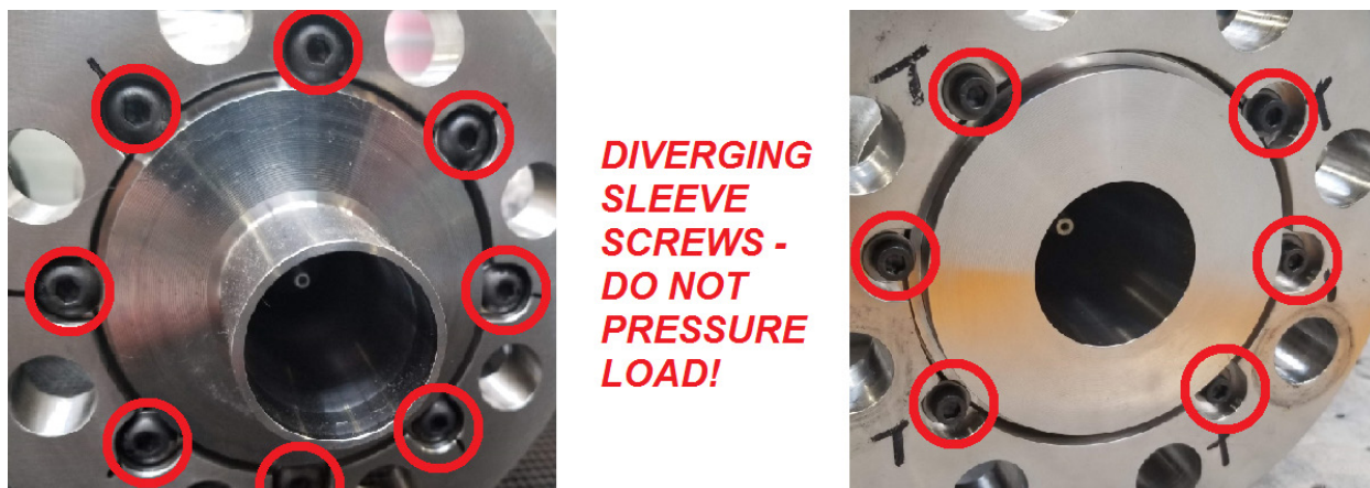
Figure 3-1. Illustration of Diverging Sleeve Screws
