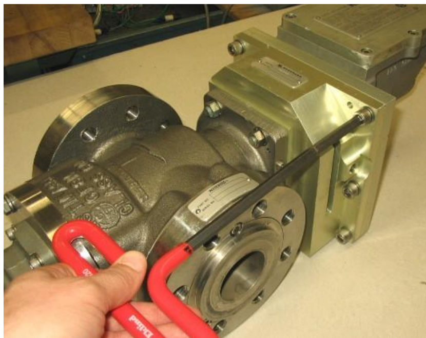
Figure 5-3. Removing Socket Head Cap Screws
