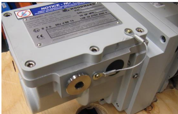
Figure 3-1. Conduit Plug (M25 Shown) & Warning Label
