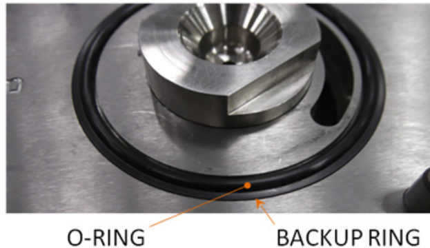
Figure 4-6. Identification O-ring and Backup Ring at Actuator-to-Manifold Interface
