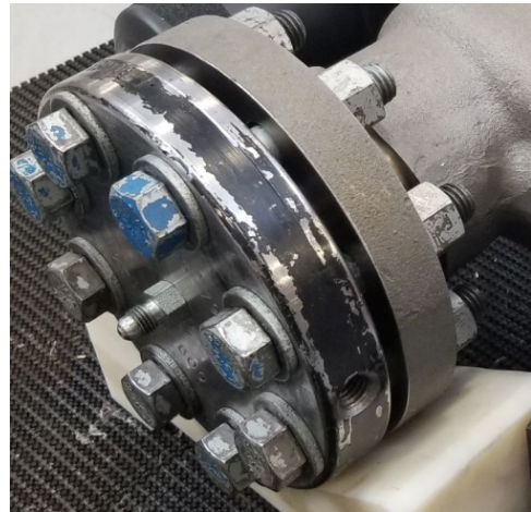
Figure 3-2. Illustration of Raised Face Style Diverging Sleeve
