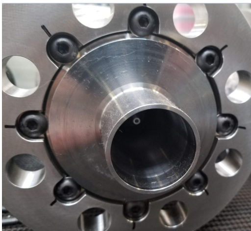
Figure 3-3. Illustration of Extension Style Diverging Sleeve
