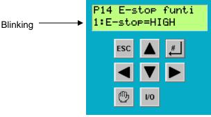
5. By using the up and down keys, set the value of P14 according to the motor type (see table below):
