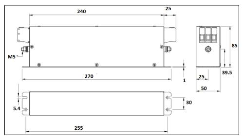
Figure 5-5. 1326-1125 Filter Assembly (mm)
