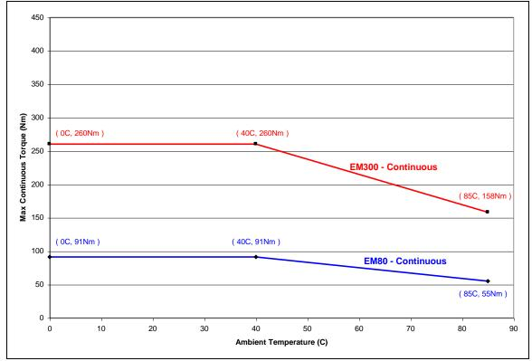
Figure 4-2. Ambient Temperature vs Torque
