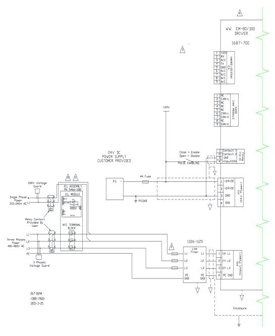
Figure 3-2a. Control Wiring Diagram (left half) (see Notes in Figure 3-2c)
