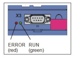
The LEDs on the front of driver give user a quick overview of the state of the driver. A green and red LED which light up in a different combination and frequencies provide information on the device's status based on a following table.
