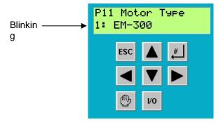
5. By using the **up and down keys** set the value of **P11** according to the motor type (see table below):
