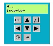
9. Navigate to the parameter **A00** using the **up and down keys** if needed, then press "**Enter key**". "0: inactive" should appear blinking on the second line of the display.
