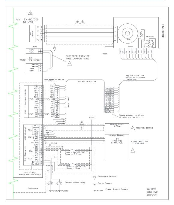
Figure 3-2b. Control Wiring Diagram (right half) (see Notes in Figure 3-2c)
