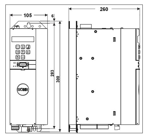
Figure 5-1. EM-80/300 Driver Dimensions (mm)
