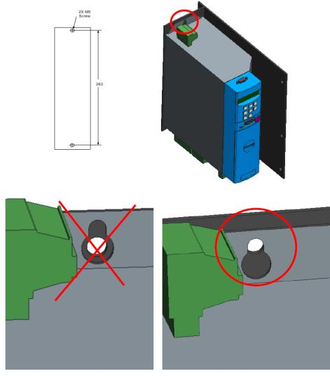
Figure 5-3. Driver Mounting Profile Dimension
