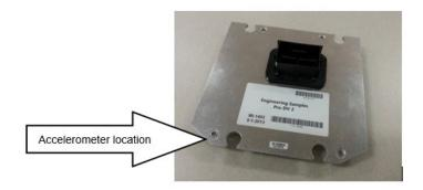
Figure 2-1. Location of Accelerometer to Measure Mounting Vibration
