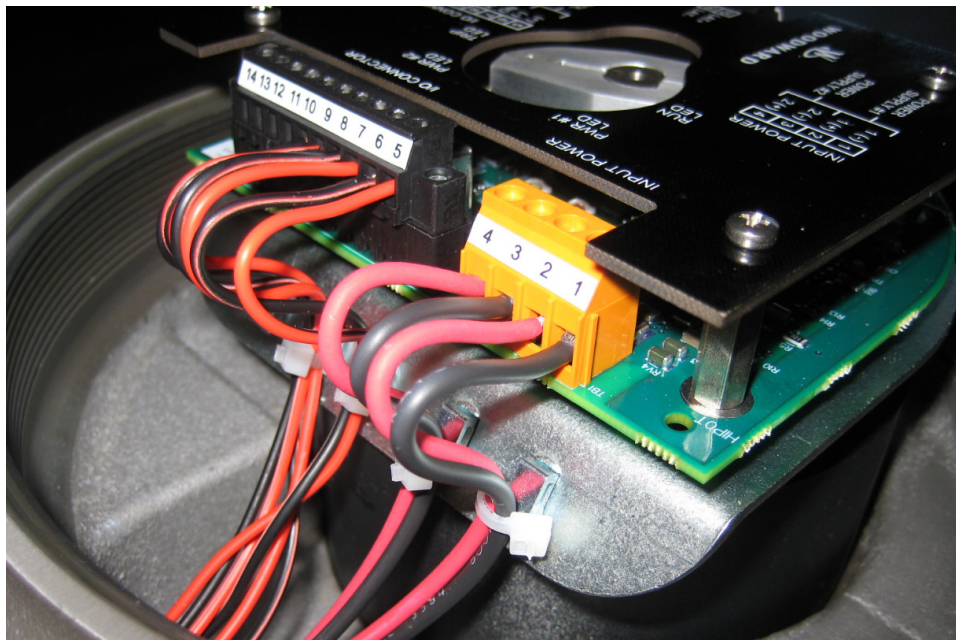
Figure 3-7. Recommended Wiring Strain Relief
