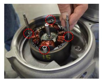
13. Gently place the electronics module (PCBA) mounting plate on top of these spacers, making sure not to knock them out of place. The rounded side of this plate must face towards the front of the QuickTrip unit (away from the conduit port).
