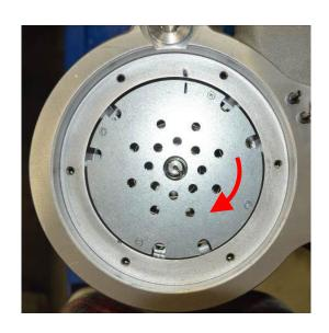
10. From this position, rotate the spring counter-clockwise as viewed from the bottom of QuickTrip (opposite from the direction of the arrow marked on the bottom of the spring assembly) so that mounting holes in the spring line up with the nearest mounting holes in the housing.
