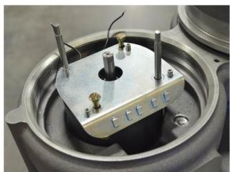
14. Re-install each of the four hex screws through the mounting plate, spacer, and solenoid, threading them into the manifold by hand. If using tool 1013-8658, only install two hex screws at this time, then torque them, per step 15 below. Then remove the two steel guide rods and install the remaining two hex screws.
