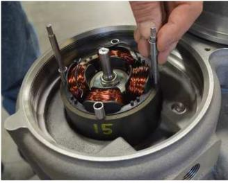
17. Gently place the electronics module (PCBA) mounting plate on top of these spacers, making sure not to knock them out of place. The rounded side of this plate must face towards the front of the QuickTrip unit (away from the conduit port).
