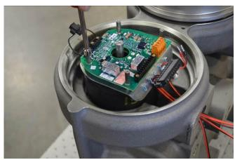
10. Plug the solenoid terminal block into the mating connector on the electronics module (TB3). Tighten the terminal block flange screws to 0.5 Nm (4.4 in-lbf) using a 2.5mm flatbladed screwdriver.
