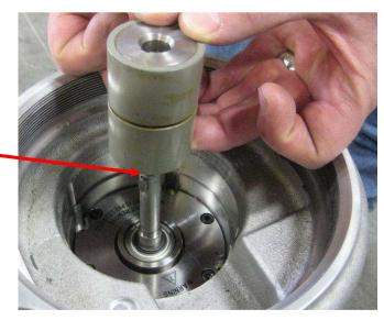
14. The rotor is a slight press fit onto the shaft. Install the washer and the hex nut and use a ¾" socket wrench to thread the nut down onto the shaft, forcing the rotor all the way onto the shaft. When the nut firmly seats against the rotor, indicating the rotor is pressed all the way onto the shaft, torque the nut to 13.5-16 Nm (10-12 ft-lbf).
