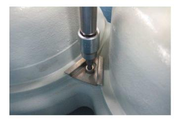
Remove electronics module cover using a spanner wrench (or Woodward tool 1013-6603).
