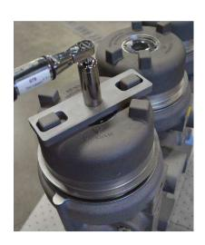
17. Re-install the cover clamp using the M5 screw using a 4mm hex driver and torque to 2-2.7 Nm (18-24 in-lbf).
