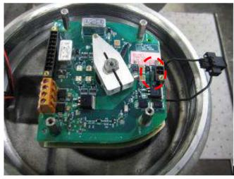
6. Remove position lever by loosening the M4 screw using a 3mm hex key.
