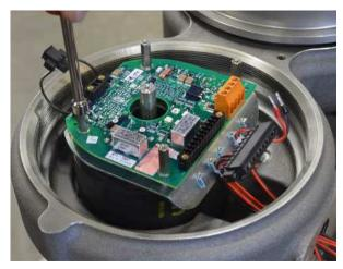
22. Note the orientation of the wires currently installed in the connector on the solenoid that was removed. Remove the pluggable connector from the old solenoid and install the wires from the new solenoid into the connector in the same orientation (wires will connect to the terminal directly above each wire and do not cross the wires).
