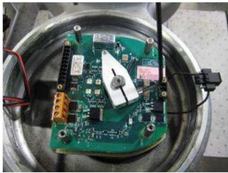
7. Remove electronics module (PCBA) by removing the four hex standoffs using a 10mm nut driver.
