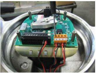
20. When wiring is complete, use plastic ratcheting wire ties to secure the wiring to the tie down points provided on the PCBA mounting plate. This helps prevent wire strain from being transmitted to the connection at the terminal block, to keep the wiring from chafing on the cover when tightening and under vibration.
