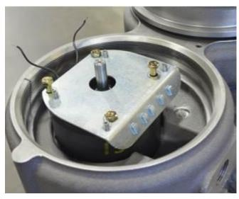
19. Torque the hex screws to 6.8-8 Nm (60-70 in-lbf) using a 10mm socket.
