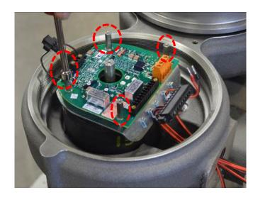
18. Note the orientation of the wires currently installed in the connector on the solenoid that was just removed. Remove the pluggable connector from the old solenoid and install the wires from the new solenoid into the connector in the same orientation (wires will connect to the terminal directly above each wire and do not cross the wires).
