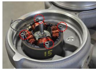
The solenoid coil may now be removed either by using the four hex screws as a handle for leverage against the magnetic attraction of the rotor or through use of Woodward Tool 1013-8658.
