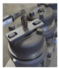
29. Re-install the cover clamp using the M5 screw using a 4mm hex driver and torque to 2-2.7 Nm (18-24 in-lbf).
