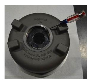
Use a spanner wrench or a specially designed tool (1013-6604) to unscrew (counter-clockwise) the sight window from the QuickTrip top cover.
