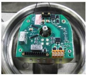
21. Secure the electronics module to the mounting plate using the four hex standoffs. Torque the standoffs to 0.3-.5 Nm (2.5-4.5 in-lbf) using a 6mm nut driver.
