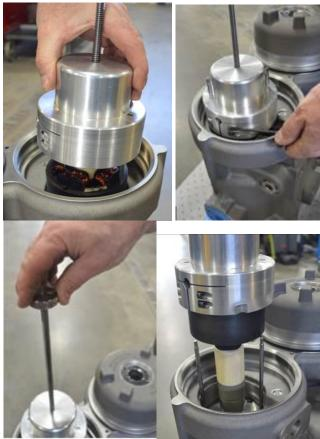
11. Remove the hex nut securing the rotor to the shaft using a ¾" socket. Remove the washer from the top of the rotor.
