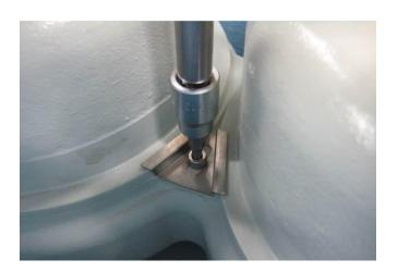
2. Remove electronics module cover using a spanner wrench (or Woodward tool 1013-6603).
