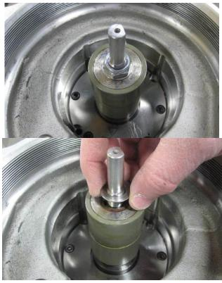
12. Remove the rotor through use of a pulley puller tool. Be sure to capture the key aligning the shaft to the rotor for re-use in the next step.
