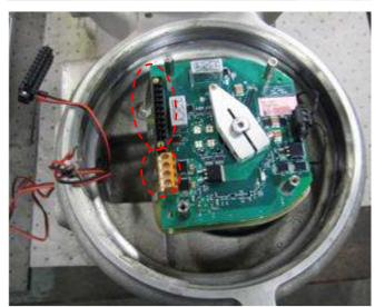
Disconnect the solenoid wiring connector (TB3) using 2.5mm flatbladed screwdriver.
