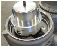
12. Place the four tubular spacers back on the outer diameter of the solenoid, making sure that each spacer is set into the semi-circular notch in the plastic flange and directly over each screw hole. If using tool 1013-8658, two spacers will go over the steel guide rods.
