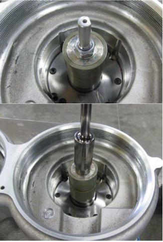
15. Re-install solenoid coil (or new solenoid coil) into housing and over rotor either by using the four hex screws as a handle for leverage against the magnetic attraction of the rotor or through use of Woodward tool 1013-8658. Ensure the two solenoid wires are facing towards the front of the unit (away from the conduit port) and that the screw holes line up with the holes in the housing. The solenoid must be completely seated within the housing.
