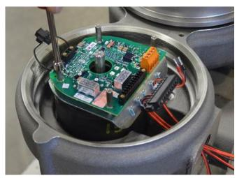
8. Place the new electronics module on top of the mounting plate, lining up the screw holes in the electronics module with the four standoffs on the mounting plate. The rounded side of the electronics module must face towards the front of the QuickTrip unit (away from the conduit port).
