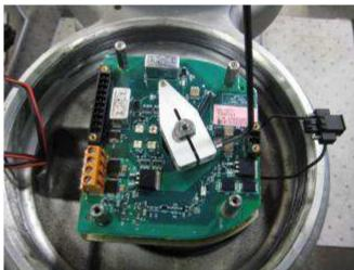
7. Remove electronics module (PCBA) by removing the four hex standoffs using a 6mm nut driver.
