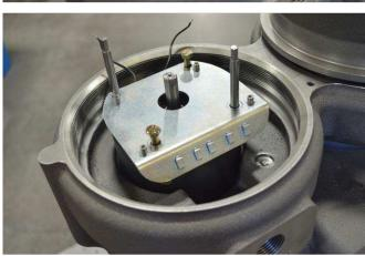
18. Re-install each of the four hex screws through the mounting plate, spacer, and solenoid, threading them into the manifold by hand. If using tool 1013-8658, only install two hex screws at this time, then torque them, per step 15 below. Remove the two steel guide rods and install the remaining two hex screws.
