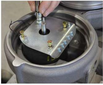
Note the position of the four tubular spacers at the outer diameter of the solenoid and remove them.
