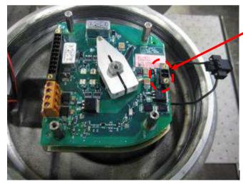
Remove position lever by loosening the M4 screw using a 3mm hex key.
