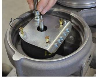
9. Note the position of the four tubular spacers at the outer diameter of the solenoid and remove them.
