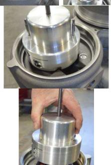
16. Place the four tubular spacers back on the outer diameter of the solenoid, making sure that each spacer is set into the semi-circular notch in the plastic flange and directly over each screw hole. If using tool 1013-8658, two of the spacers will be installed over the steel guide rods.
