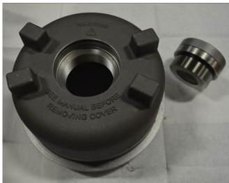
4. Make sure the O-ring seal is installed on the sight glass housing just under the top flange.
