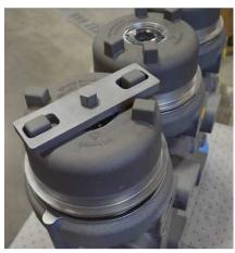
Remove top silkscreen wiring diagram cover by removing the four Philips screws.
