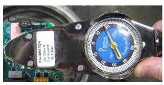
13. Re-install the bottom cover, ensuring the O-ring is carefully seated in the O-ring groove. Install the six M5 screws and torque to 3.1-3.8 Nm (28-34 in-lbf).
