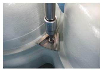
Remove electronics module cover using a spanner wrench (or Woodward tool 1013-6603). Make sure the O-ring is still installed on the cover, as it will be reused. If the O-ring is damaged, the top cover replacement kit contains a replacement O-ring.
