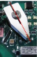
22. Re-install the silkscreen wiring diagram cover by placing it onto the hex standoffs, lining up the four holes in the cover with the four standoffs. The rounded side of the cover should face towards the front of the QuickTrip unit (away from the conduit port).
