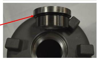
Re-install the sight window by carefully threading it into the QuickTrip top cover (clockwise). Use a spanner wrench or specially designed tool (1013-6604) to tighten the sight glass into the cover, making sure not to crossthread or otherwise damage the threads.
