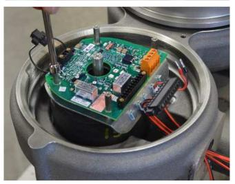
Remove the electronics module (PCBA) mounting plate by removing the four hex screws using a 10mm socket.
