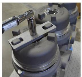
25. Re-install the cover clamp with M5 screw using a 4mm hex driver and torque to 2-2.7 Nm (18-24 in-lbf).
