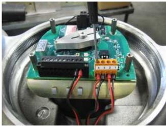
24. When wiring is complete, use plastic ratcheting wire ties to secure the wiring to the tie down points provided on the PCBA mounting plate. This helps prevent wire strain from being transmitted to the connection at the terminal block and to keep the wiring from chafing on the cover when tightening and under vibration.
