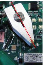
22. Re-install the silkscreen wiring diagram cover by placing it onto the hex standoffs, lining up the four holes in the cover with the four standoffs. The rounded side of the cover should face towards the front of the QuickTrip unit (away from the conduit port).
