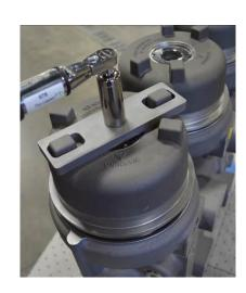
17. Re-install the cover clamp using the M5 screw using a 4mm hex driver and torque to 2-2.7 Nm (18-24 in-lbf).
