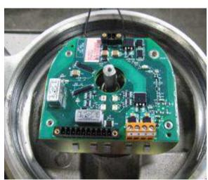
17. Secure the electronics module to the mounting plate using the four hex standoffs. Torque the standoffs to 0.3-.5 Nm (2.5-4.5 inlbf) using a 6mm nut driver.
