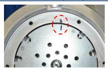
9. Rotate the spring clockwise approximately 1-3/4 turns, either by hand or by using Woodward tool 1013-8795, as viewed from the bottom of QuickTrip (in the direction of the arrow marked on the bottom of the spring assembly). Use the marks from the previous step as a reference for winding the spring.
