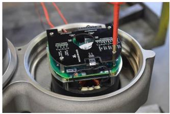
Disconnect the customer interface cable connections from PCB (TB1 and TB2) using a 2.5mm flat-bladed screwdriver.
