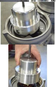
16. Place the four tubular spacers back on the outer diameter of the solenoid, making sure that each spacer is set into the semi-circular notch in the plastic flange and directly over each screw hole. If using tool 1013-8658, two of the spacers will be installed over the steel guide rods.
