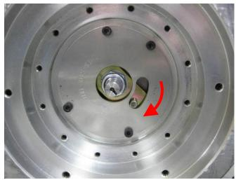
7. Install the new return spring, inserting spring "tang" into slot in shaft, ensuring lettering "WIND DIRECTION" and arrow are visible and facing down (unit orientation).
