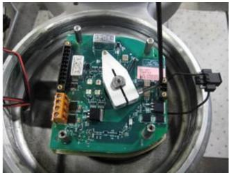
7. Remove electronics module (PCBA) by removing the four hex standoffs using a 10mm nut driver.
