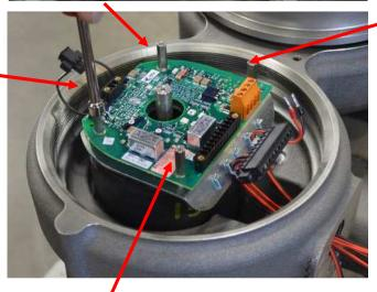
8. Remove the electronics module (PCBA) mounting plate by removing the four hex screws using a 10mm socket.
