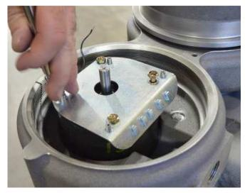
16. Place the electronics module on top of the mounting plate, lining up the screw holes in the electronics module with the four standoffs on the mounting plate. The rounded side of the electronics module must face towards the front of the QuickTrip unit (away from the conduit port).
