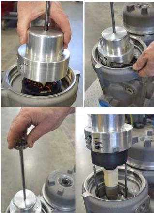
11. Remove the hex nut securing the rotor to the shaft using a 3/4" socket. Remove the washer from the top of the rotor.
