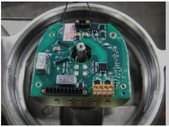
Secure the electronics module to the mounting plate using the four hex standoffs. Torque the standoffs to 0.3-.5 Nm (2.5-4.5 in-lbf) using a 6mm nut driver.
