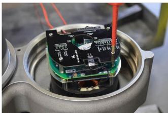
4. Disconnect the customer interface cable connections from PCB (TB1 and TB2) using 2.5mm flat-bladed screwdriver.
