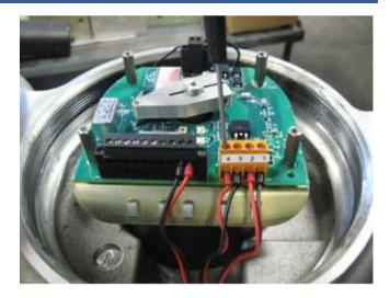
12. When wiring is complete, use plastic ratcheting wire ties to secure the wiring to the tie down points provided on the PCBA mounting plate. This helps prevent wire strain from being transmitted to the connection at the terminal block, to keep the wiring from chafing on the cover when tightening and under vibration.
