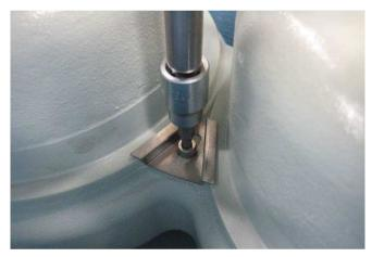
Remove electronics module cover using a spanner wrench (or Woodward tool 1013-6603). Make sure the O-ring is still installed on the cover, as it will be reused. If the O-ring is damaged, the top cover replacement kit contains a replacement O-ring.
