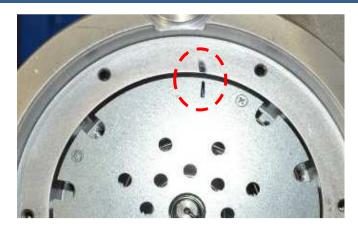
9. Rotate the spring clockwise approximately 1-3/4 turns, either by hand or by using Woodward tool 1013-8795, as viewed from the bottom of QuickTrip (in the direction of the arrow marked on the bottom of the spring assembly). Use the marks from the previous step as a reference for winding the spring.
