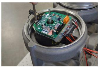
Plug the solenoid terminal block into the mating connector on the electronics module (TB3). Tighten the terminal block flange screws to 0.5 Nm (4.4 in-lbf) using a 2.5mm flatbladed screwdriver.
