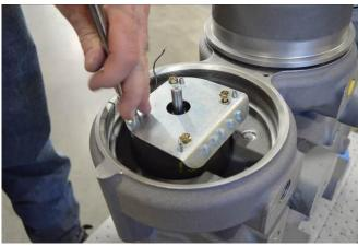
20. Place the electronics module on top of the mounting plate, lining up the screw holes in the electronics module with the four standoffs on the mounting plate. The rounded side of the electronics module must face towards the front of the QuickTrip unit (away from the conduit port).
