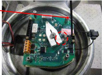
7. Remove electronics module (PCBA) by removing the four hex standoffs using a 6mm nut driver.
