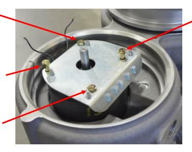
15. Torque the hex screws to 6.8-8 Nm (60-70 in-lbf) using a 10mm socket.
