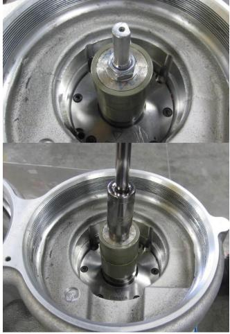
15. Re-install solenoid coil (or new solenoid coil) into housing and over rotor either by using the four hex screws as a handle for leverage against the magnetic attraction of the rotor or through use of Woodward tool 1013-8658. Ensure the two solenoid wires are facing towards the front of the unit (away from the conduit port) and that the screw holes line up with the holes in the housing. The solenoid must be completely seated within the housing.
