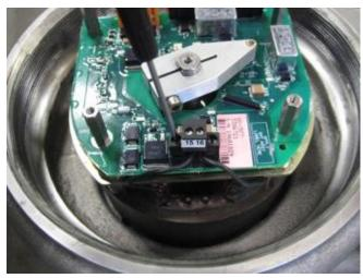
11. Re-install the customer interface cable connections to the electronics module (TB1 and TB2). Tighten the terminal block flange screws to 0.5 Nm (4.4 in-lbf) using a 2.5mm flatbladed screwdriver.
