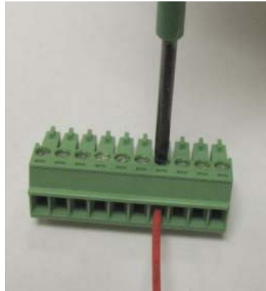
Figure 5-2. Screw Connection Terminal Block Used on A5200 SmartCore Board
