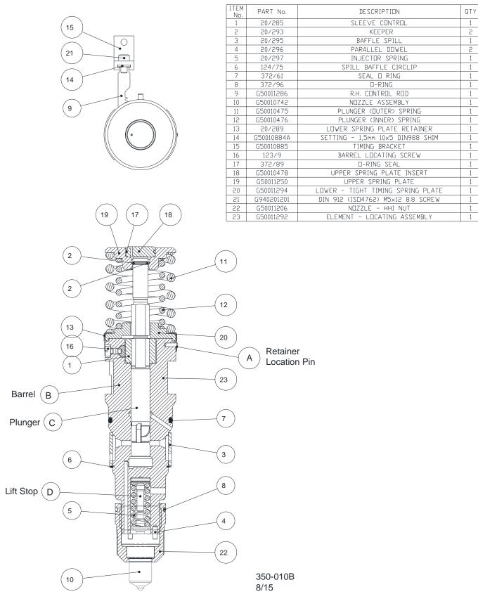
Figure 4-2. Type G50011293 Unit Injector
