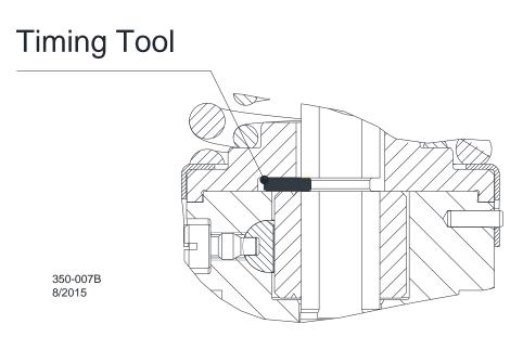
Figure 7-1. Use of Timing Tool to Locate Plunger
