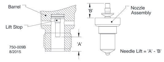
Figure 6-1. Needle Lift Dimension
