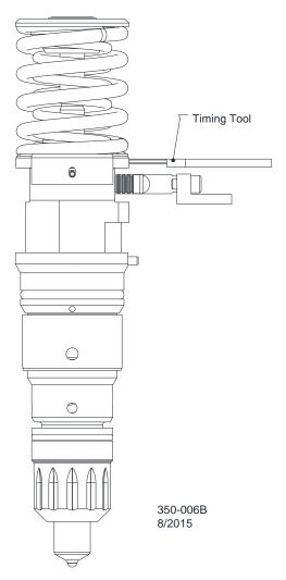
Figure 2-1. G50011293 Unit Injector
