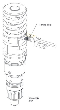
Figure 1-1. G50011293 Unit Injector
