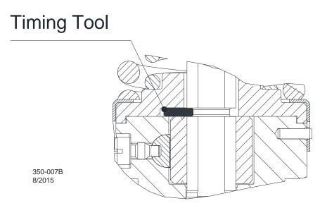
Figure 4-1. Use of Gauge Tool to Fix Plunger Position
