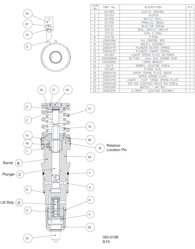
Figure 7-2. Type G50011293 Unit Injector
