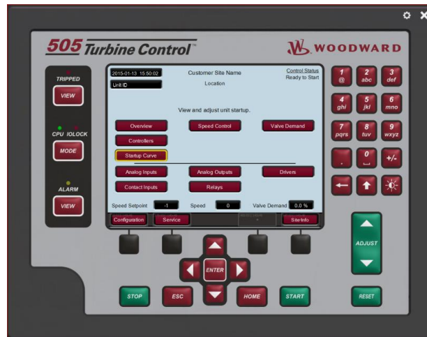
Figure 5-26. HOME Menu Showing “Startup Curve” IN-Focus
