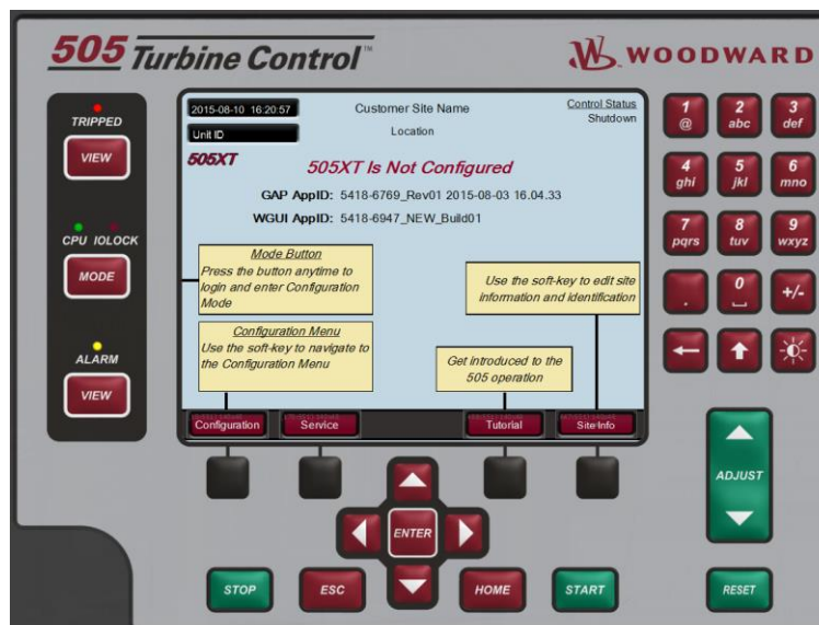
Figure 4-1. Initial HOME Screen (Unit Not Configured)
