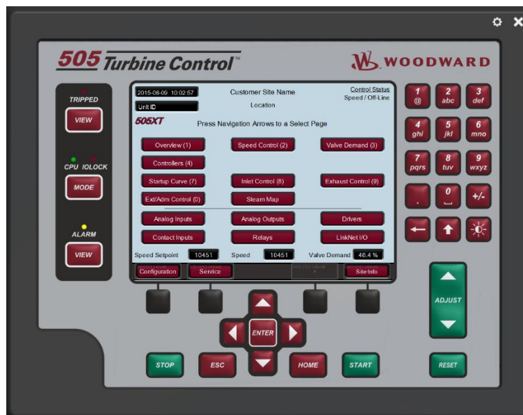
Figure 1-10. 505 Keypad and Display
