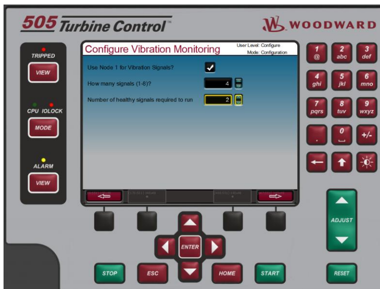
Figure 1-7. Vibration Wizard for LinkNet Node 1
