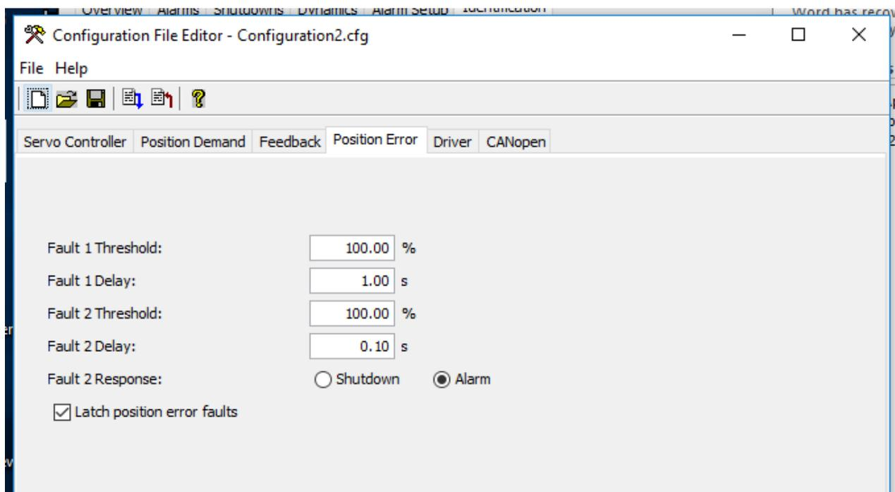
Figure 2-15e. SPC Driver Configuration for Redundant Actuators
