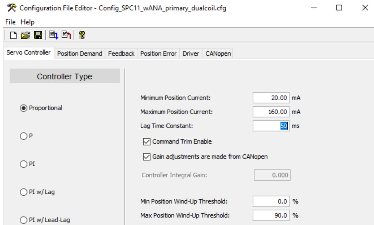
Figure 2-15a. SPC Driver Configuration for Redundant Actuators
