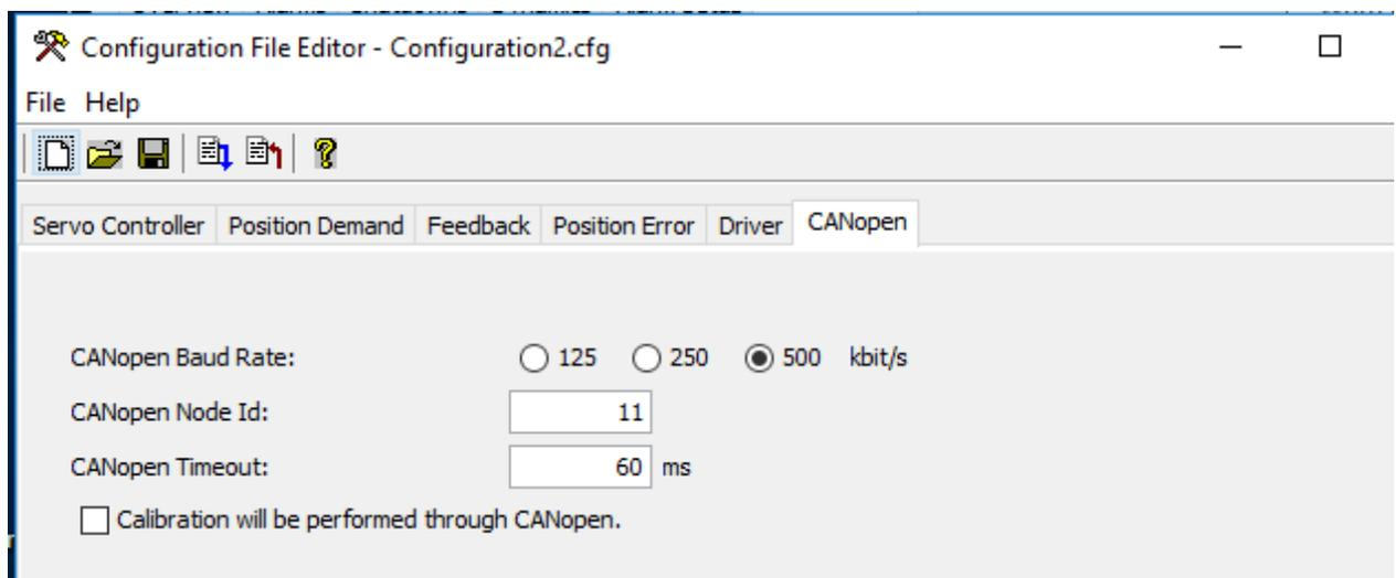
Figure 2-15g. SPC Driver Configuration for Redundant Actuators
