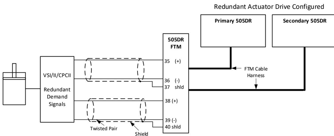
Figure 2-8. Actuator Driver with Redundant Demands
