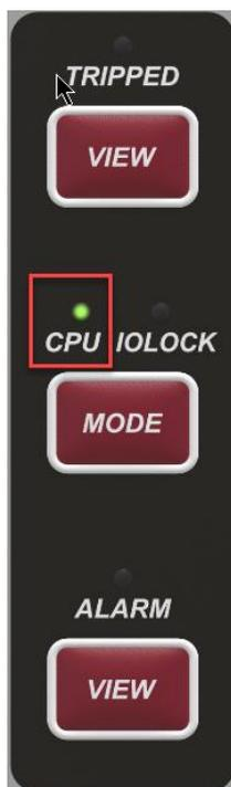
Figure 3-5. Front Panel CPU LED SYCON/BACKUP Indication
