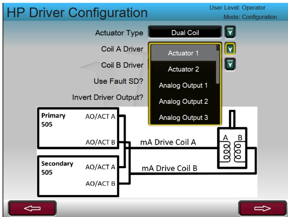
Figure 2-10. Driver Channel Configuration
