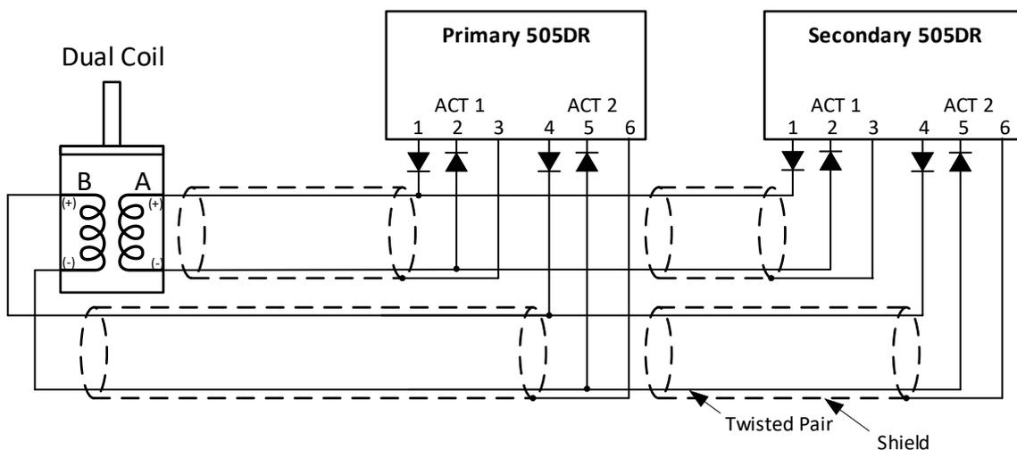
Figure 2-4. Dual Coil Driver
