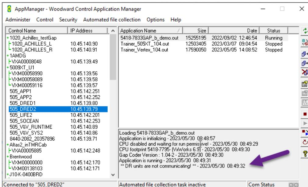
Figure 4-3. AppManager Status – No Interlock Wiring
