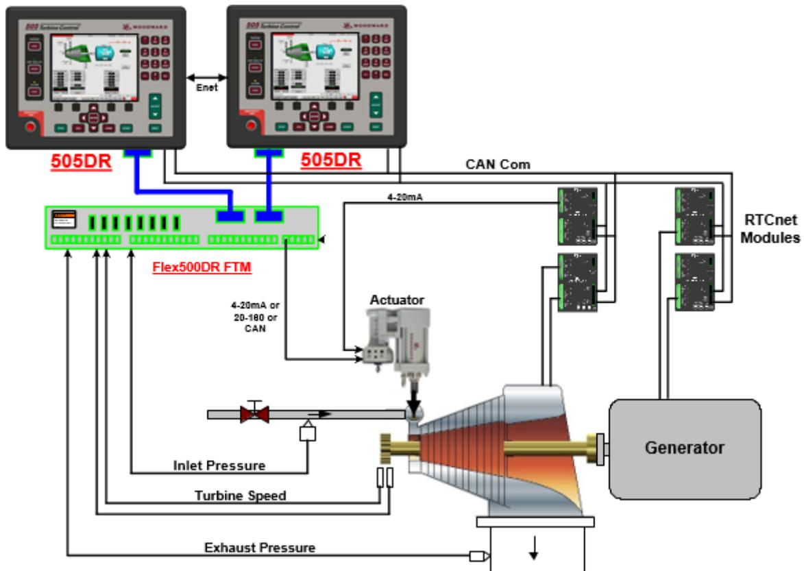
Figure 1-1. Typical Redundant 505XT Application Configuration
