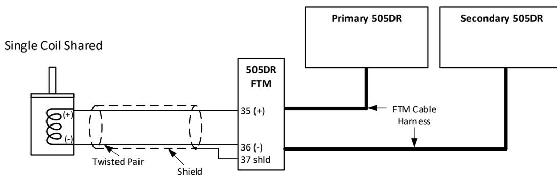
Figure 2-3. Single Coil Shared Driver with 505DR FTM
