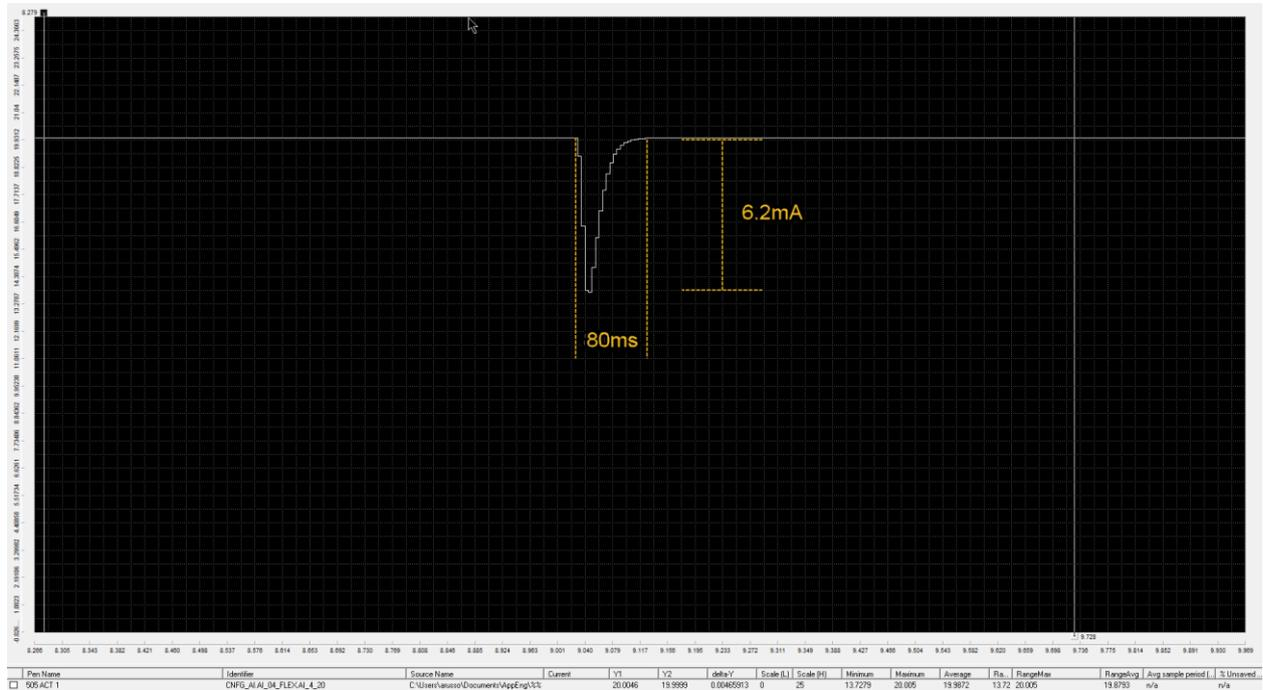
Figure 3-23. Actuator Output Failover Performance
