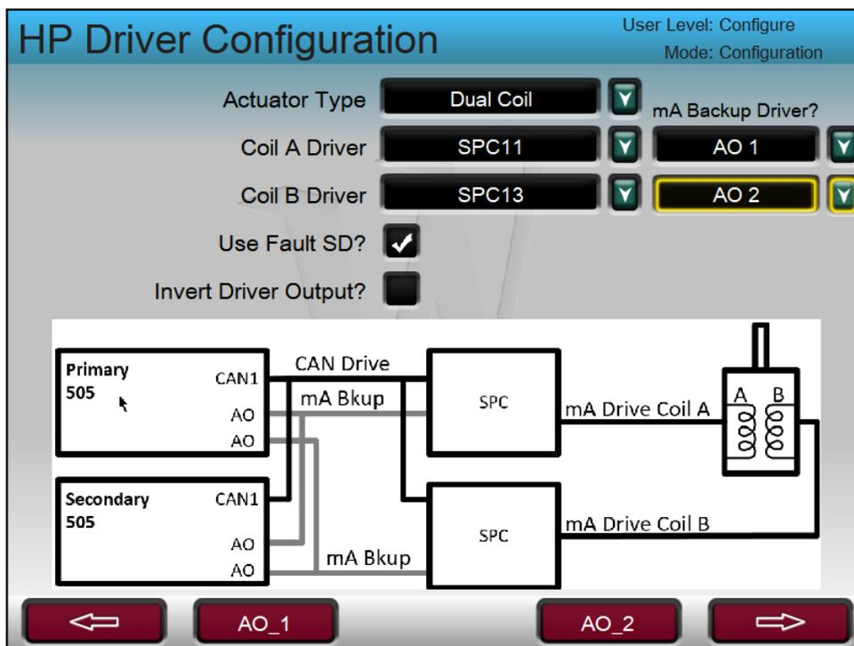
Figure 2-11. mA Backup Channel Configuration
