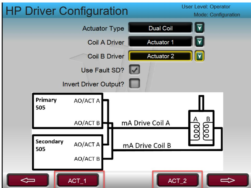
Figure 2-12. Driver Configuration Page Buttons
