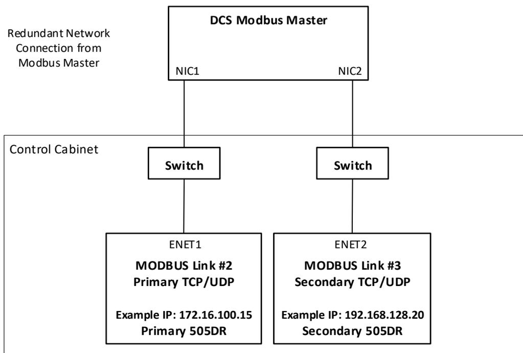
Figure 2-19. Redundant Network Modbus Architecture
