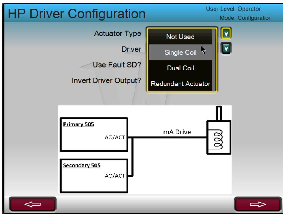
Figure 2-9. Actuator Type Configuration
