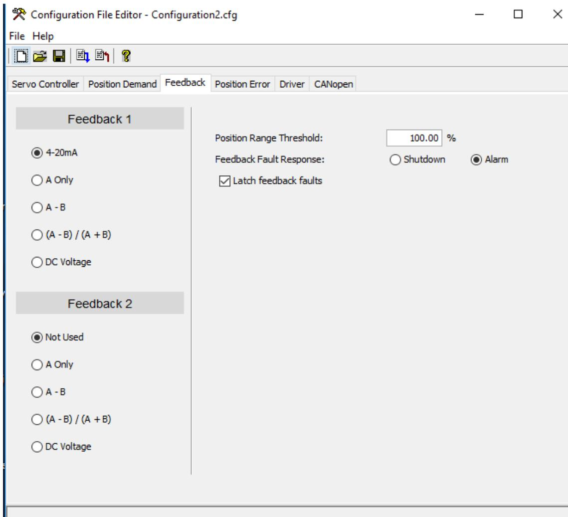
Figure 2-15d. SPC Driver Configuration for Redundant Actuators
