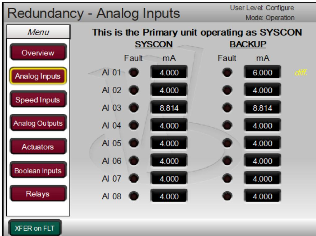
Figure 3-10. BACKUP Analog Inputs Screen
