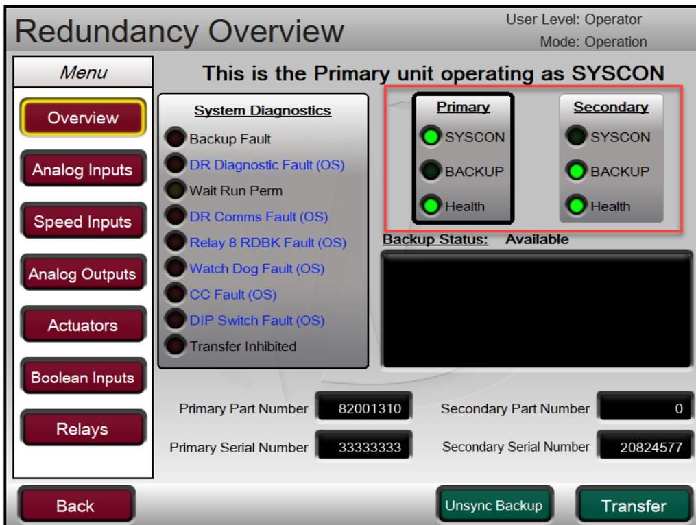
Figure 3-4. Primary/Secondary SYSCON/BACKUP Indications
