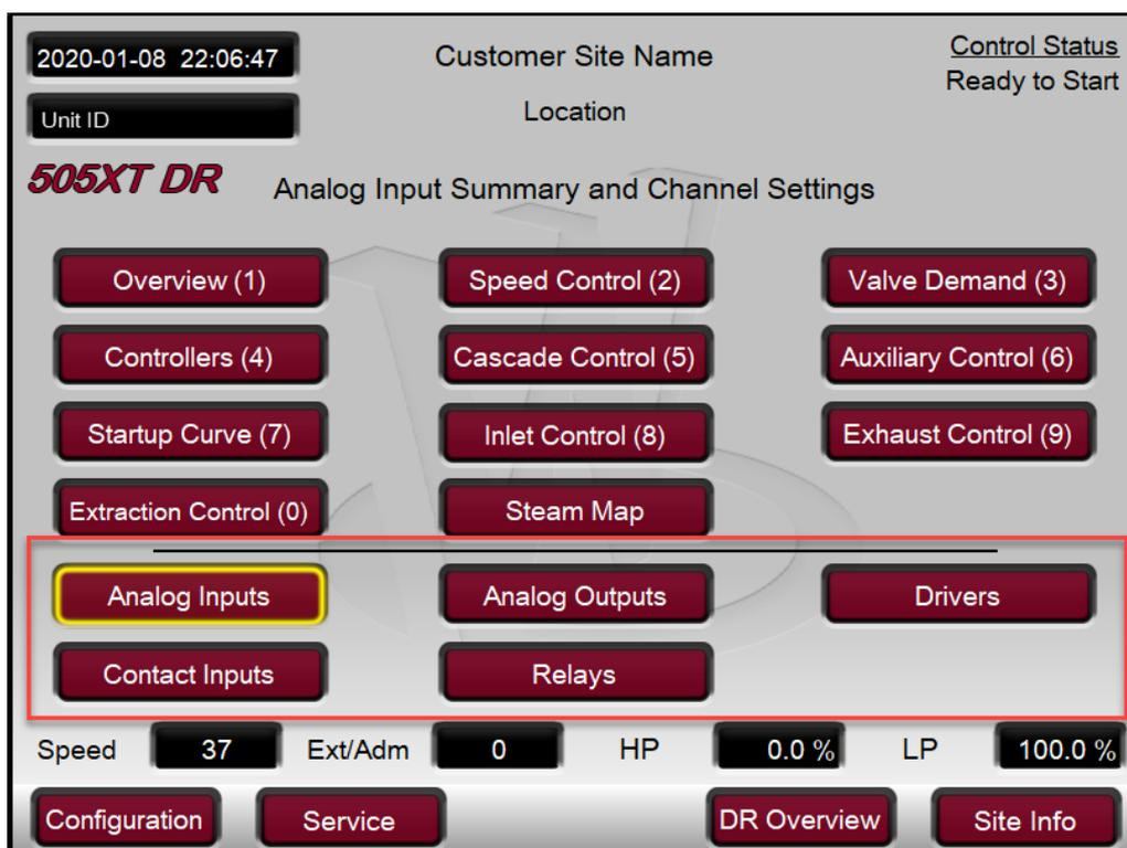
Figure 3-6. SYSCON I/O Monitoring Pages
