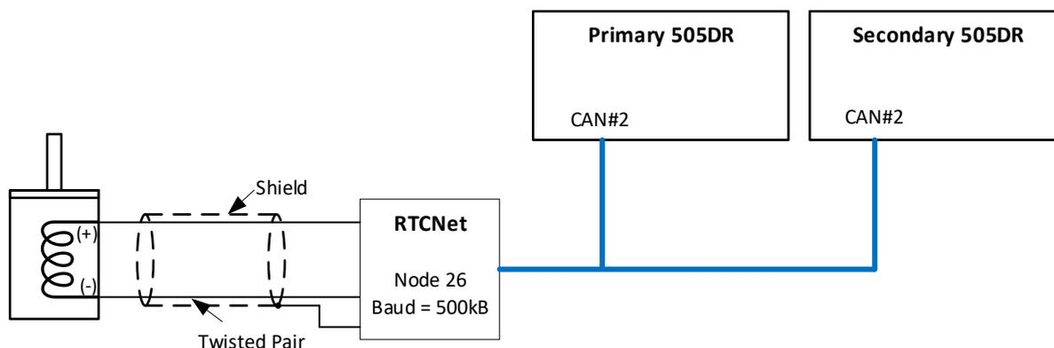
Figure 2-17. Expandable I/O Node 26 Driver (Bumpless SYSCON Transfer)
