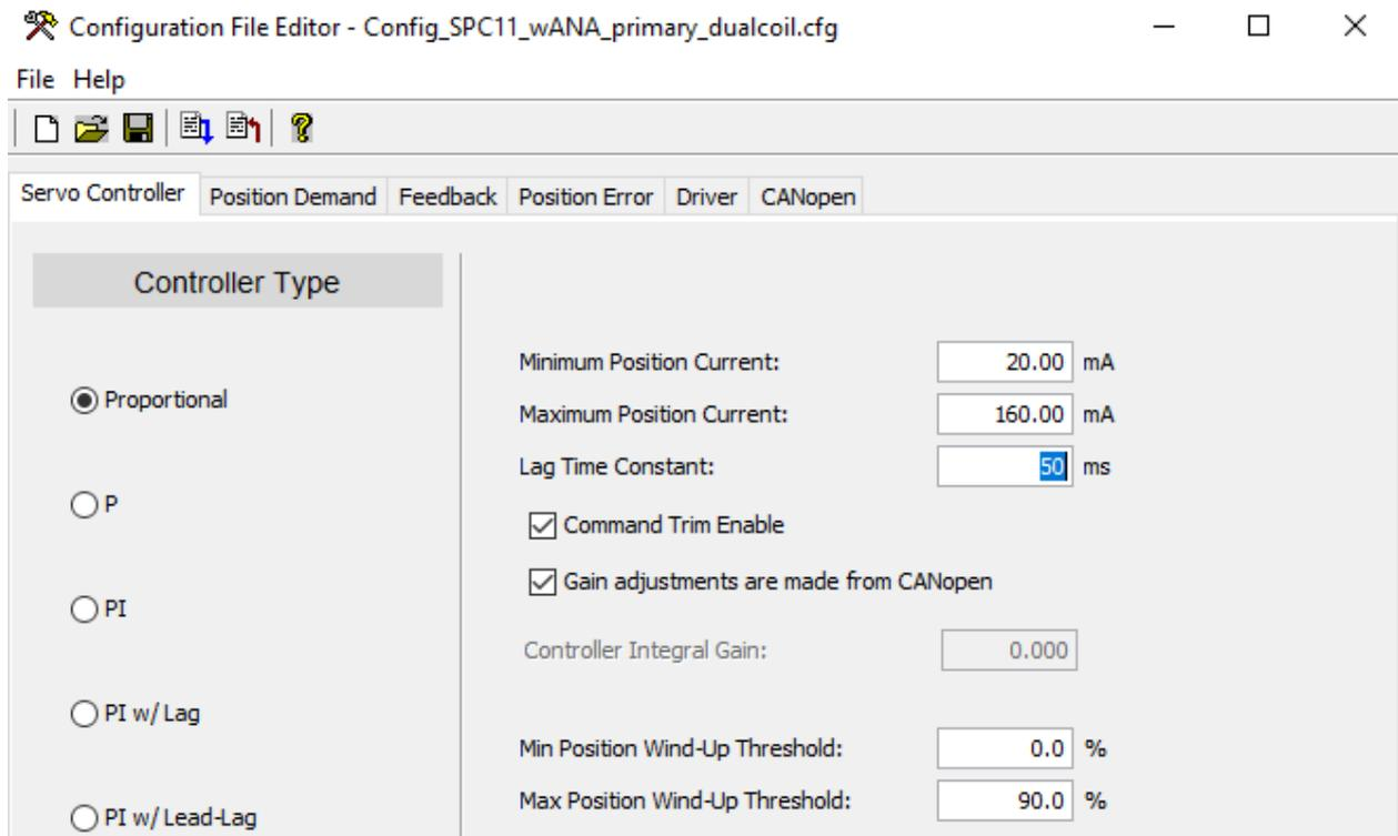
Figure 2-16a. SPC Driver Configuration for Dual Coil Actuators
