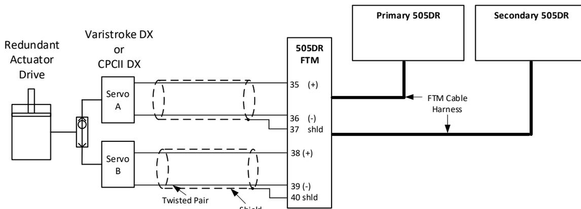
Figure 2-7. Redundant (Parallel) Actuator Driver with 505DR FTM
