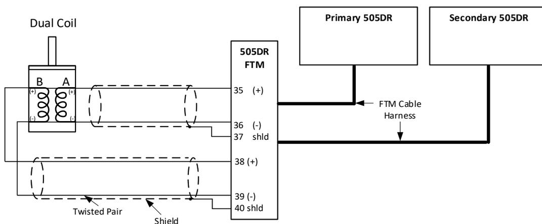
Figure 2-5. Dual Coil Driver with 505DR FTM
