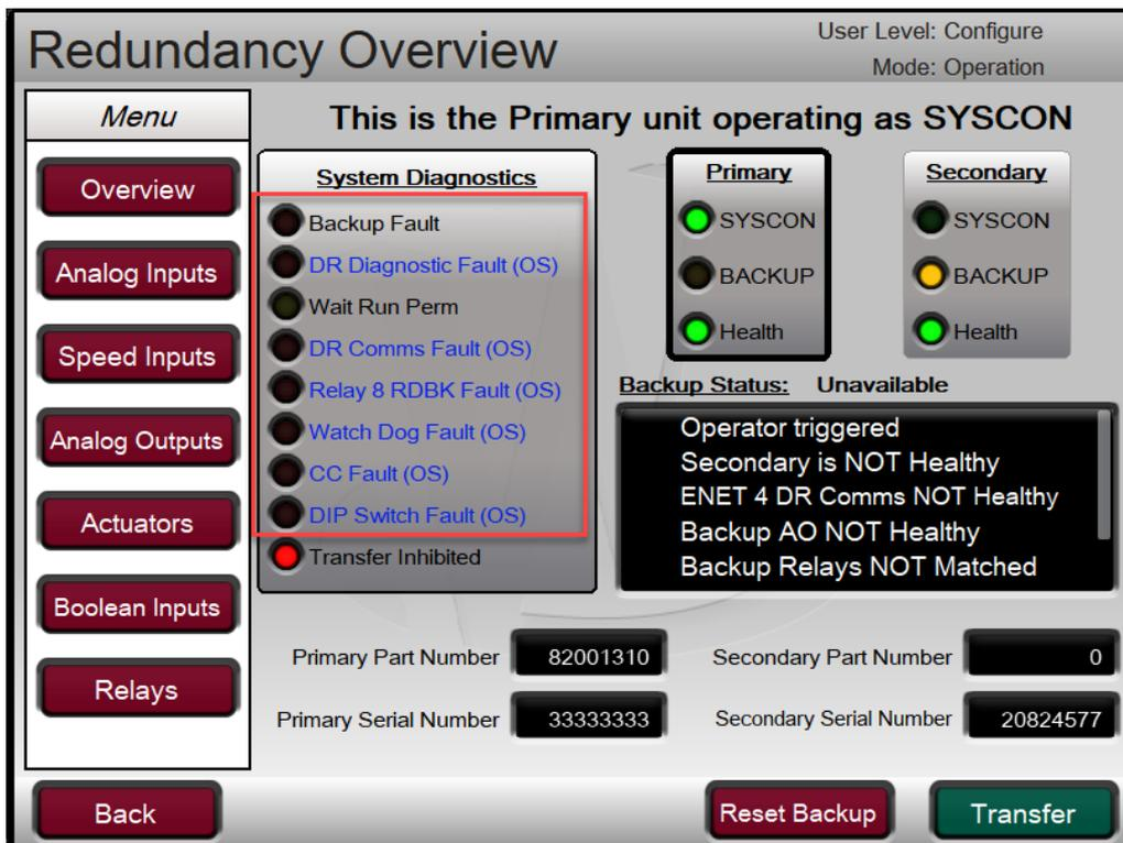
Figure 3-20. System Diagnostic Faults Cleared
