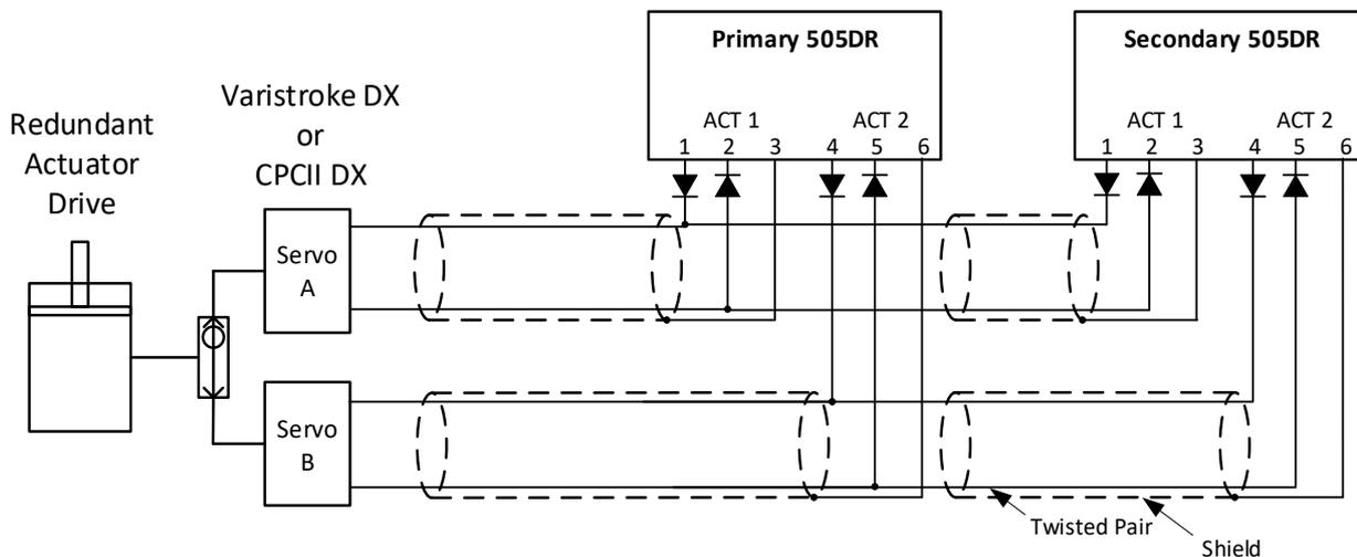
Figure 2-6. Redundant (Parallel) Actuator Driver
