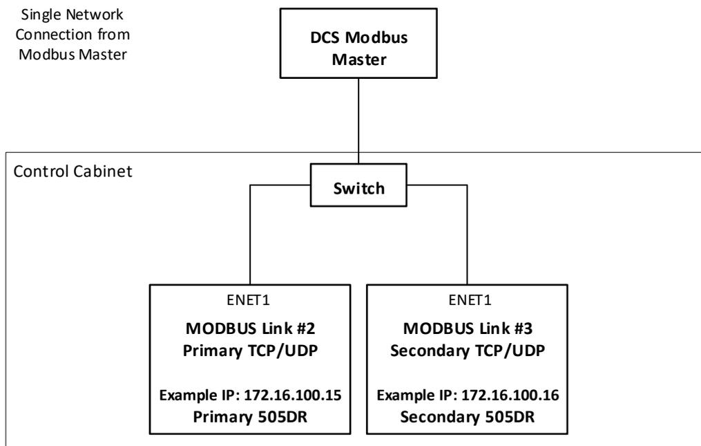
Figure 2-18. Single Network Modbus Architecture
