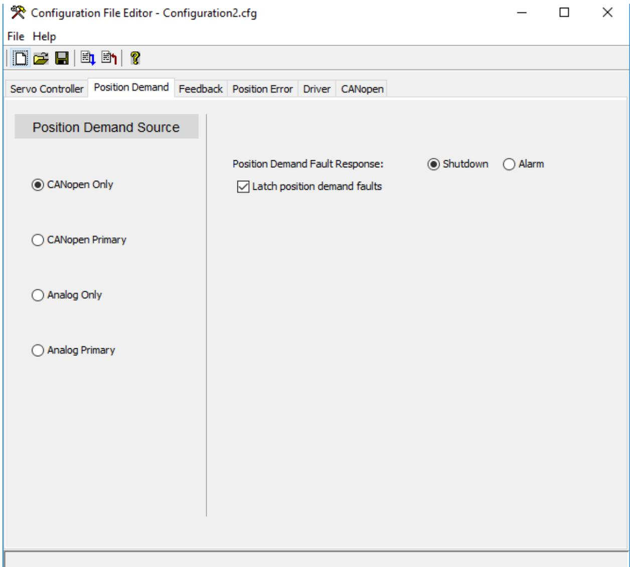
Figure 2-15b. SPC Driver Configuration for Redundant Actuators
