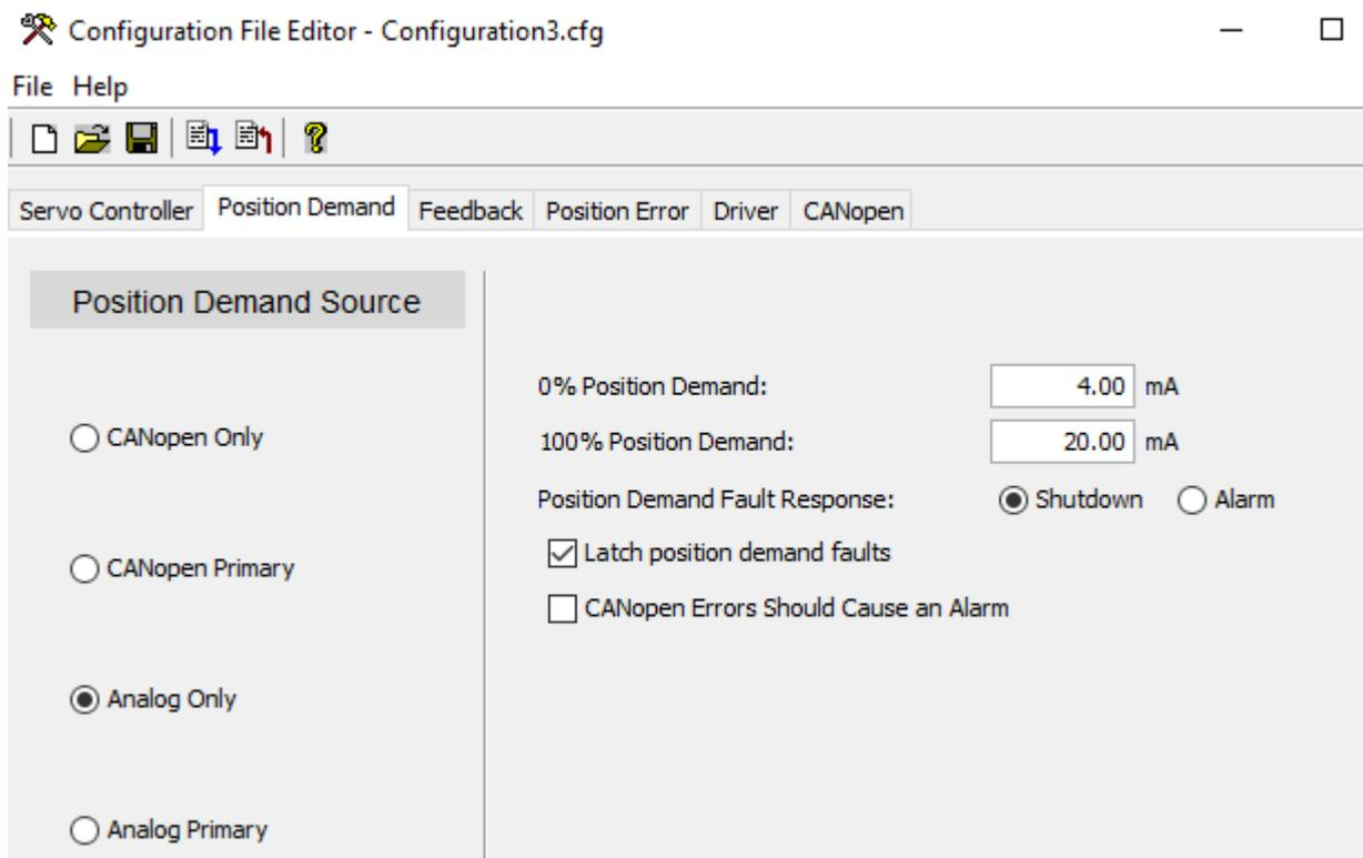
Figure 2-16b. SPC Driver Configuration for Dual Coil Actuators
