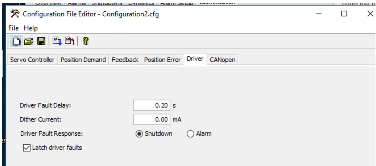
Figure 2-15f. SPC Driver Configuration for Redundant Actuators
