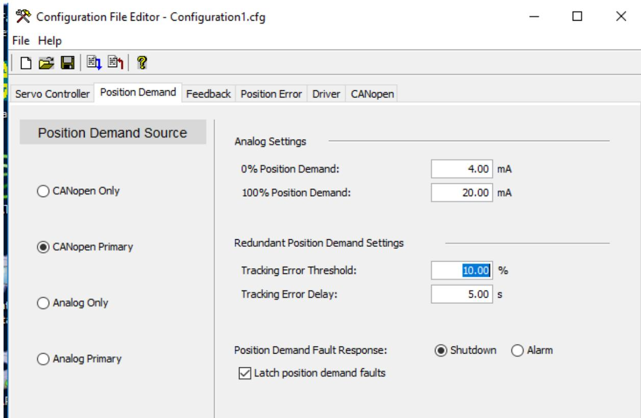
Figure 2-15c. SPC Driver Configuration for Redundant Actuators
