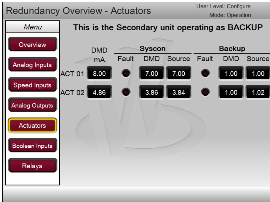
Figure 3-13. BACKUP Actuator Outputs Screen
