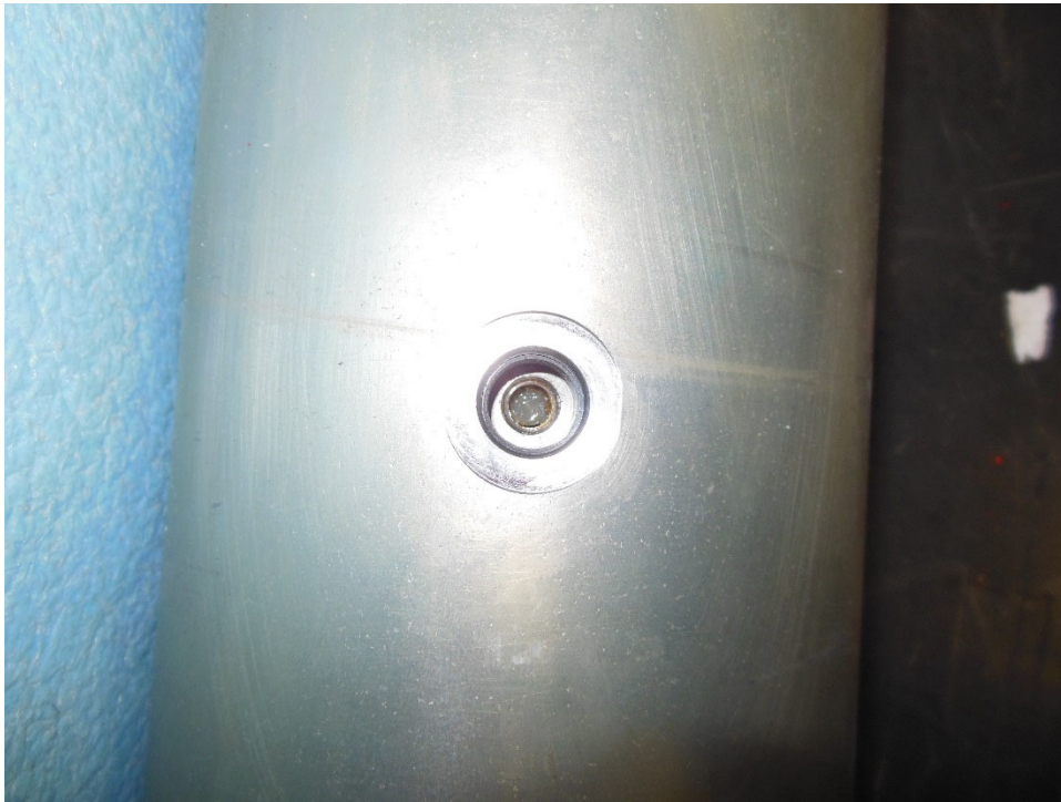
Figure 1-7. Body Grease Port Unplugged
