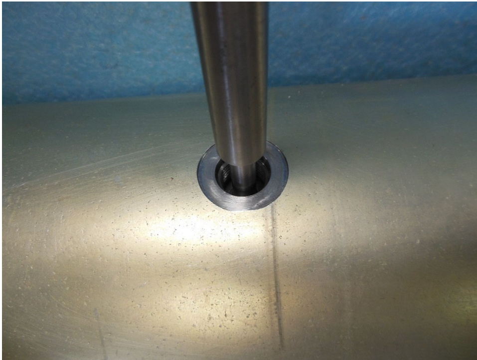
Figure 1-8. Body Grease Port with Greasing Adaptor Installed
