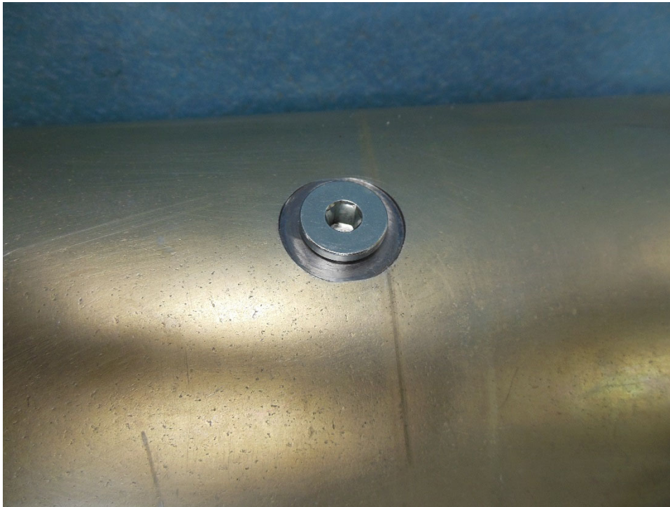
Figure 1-5. Actuator Body Grease Port with Plug Installed
