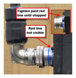
Figure 3-3. Motor Resolver Connectors
