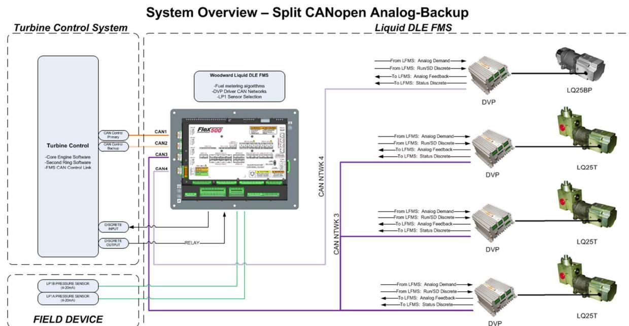
Figure 3-2. LFMS System Overview Split CANopen (Mode Config=2)
