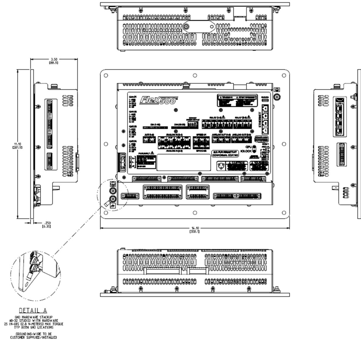
Figure 3-3c. Flex500 Bulkhead Envelope Dimensions and Grounding details
