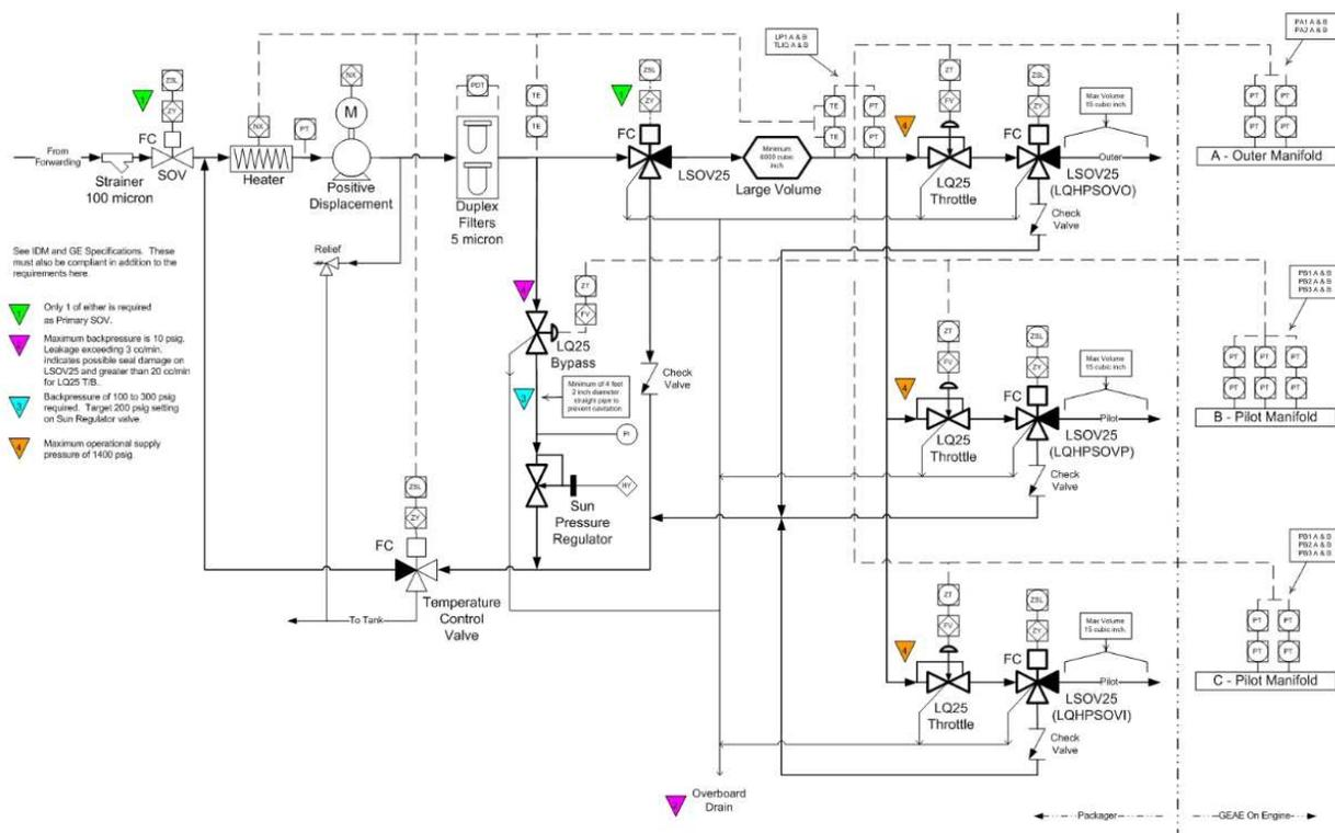
Figure 2-1. Liquid Fuel System P&ID
