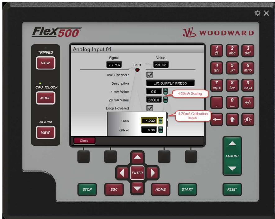
Figure 6-5. Analog Input Channel Configuration
