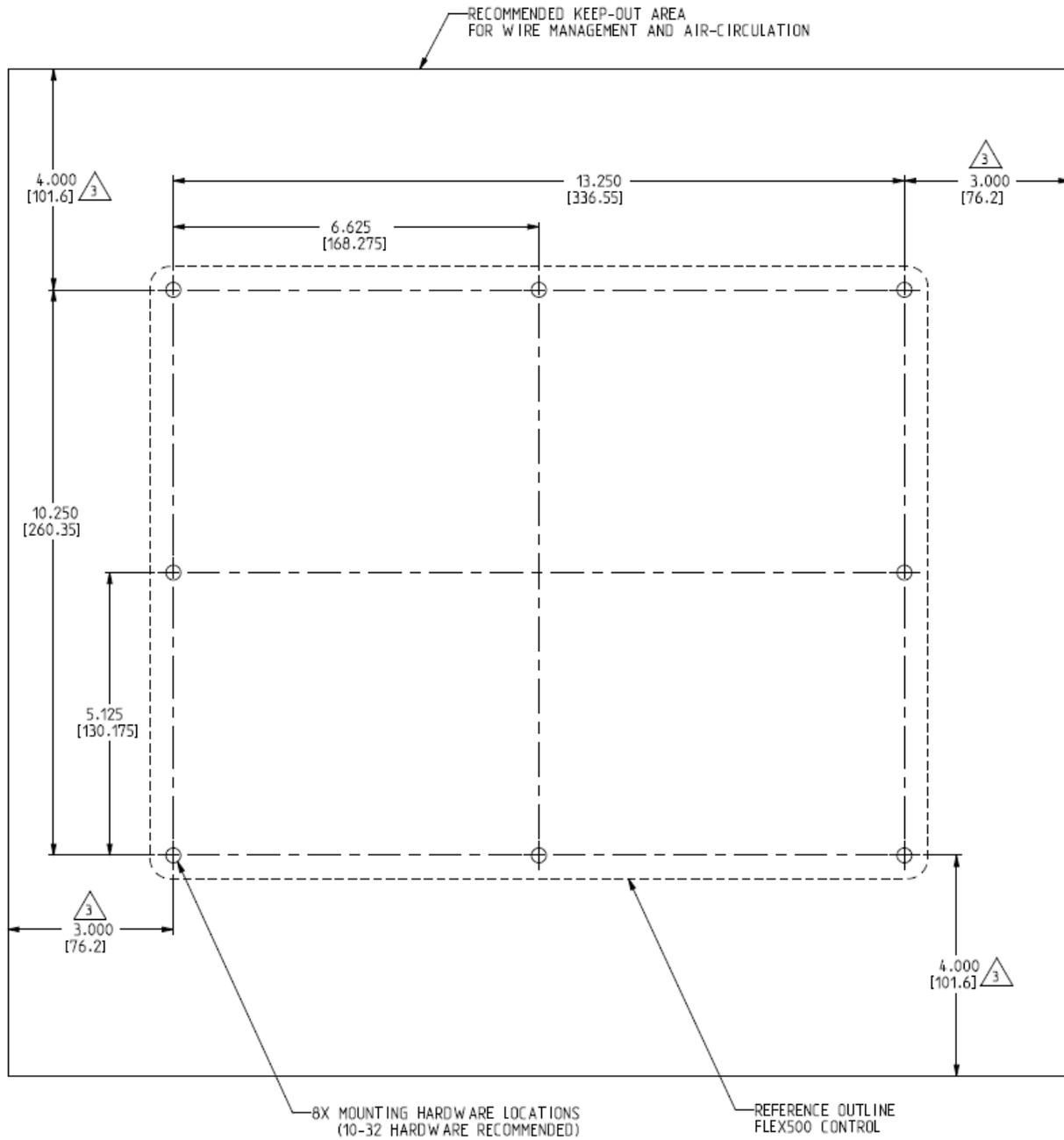
Figure 3-3b. Flex500 Bulkhead Panel Mounting Reference
