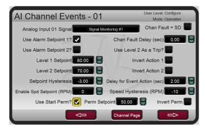
Figure I-13. Menu Selection for Analog Input Start Permissive
