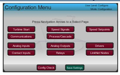
Figure 3-8. Configuration Menu – Configuration Mode (Edit)
