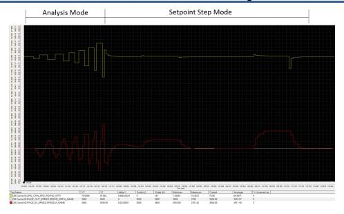
Figure C-2. Speed vs Actuator Trends During Analysis
