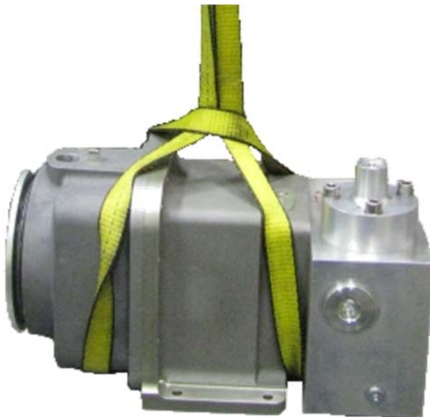
Figure 2-2. Using a Sling to Lift the Valve
