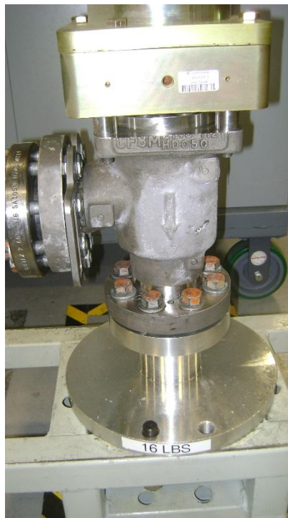
Figure 3-6. Support Flange Bolted to Outlet Flange
