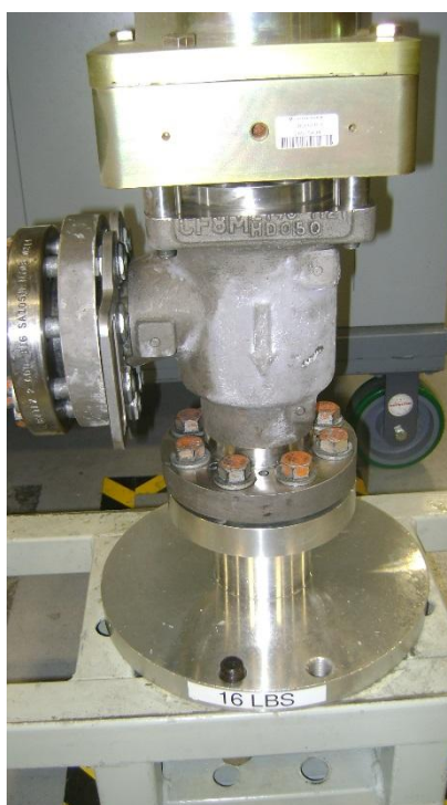
Figure 3-6. Support Flange Bolted to Outlet Flange
