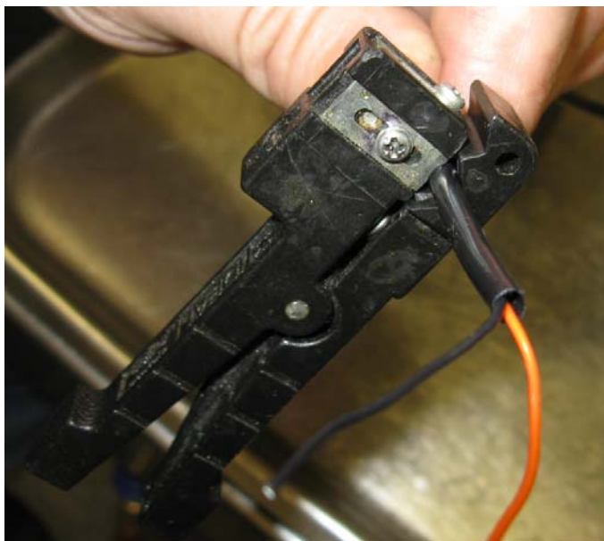
Figure 7. Trim Back Existing Hard Bundle Sheathing
