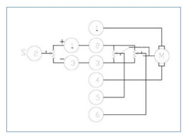
Figure 1. Electronic Throttle/Slider Potentiometer Schematic
