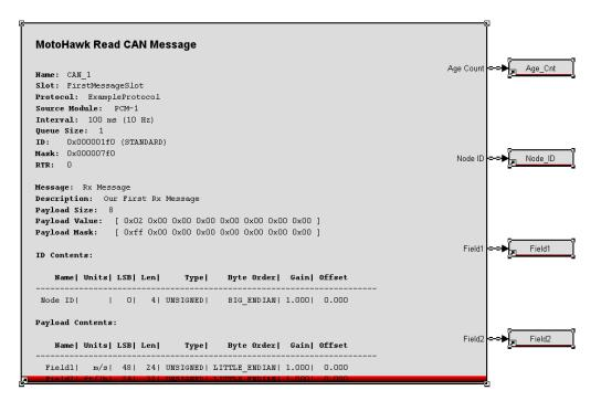
6. Note the 1F3 message being transmitted. The 3 comes from the Node ID input.
