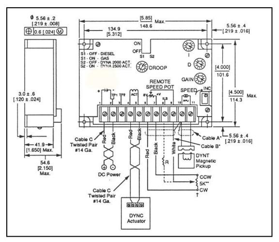
Figure 1. Electronic Control Box Adjustments, Configuration and Typical Wiring Diagram
