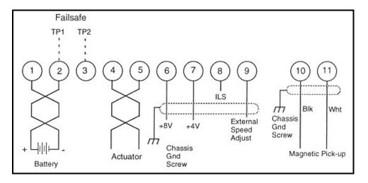
Figure 2. Typical Wiring for CE Models
