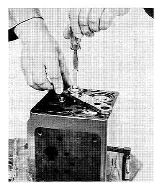
Figure 4-2. Removal of Check Valves
