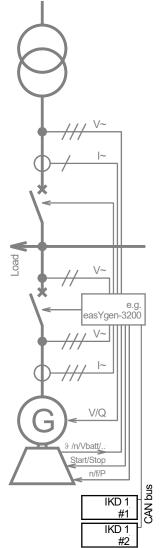
The digital inputs are read by the IKD 1 and transferred via the CAN bus to the control unit (incl. alarm class). Each alarm input may have a delay as well as the control logic (NO/NC) configured individually during set up. The status of the alarm input is monitored in the control device and will show the alarm text in its display. The alarm class assigned in the control device evaluates the alarm input and reacts accordingly.
