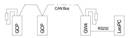
Observe the notes about termination (termination resistor) of the CAN bus under Connection on page 5. Up to 4 GCPs can be connected to a GW 4.
