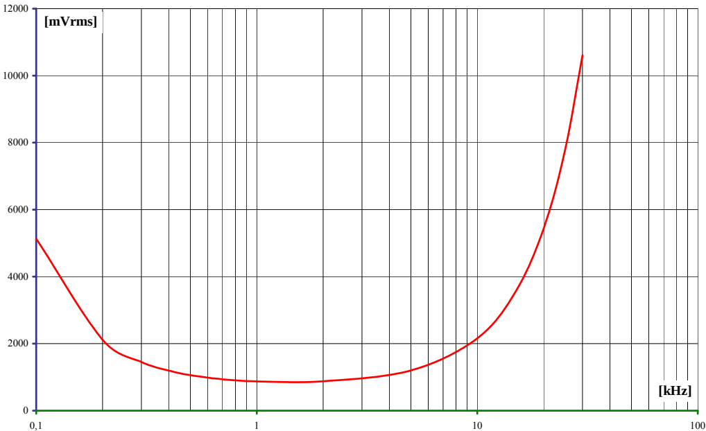
Figure 6-31: Minimal necessary input voltage depending on frequency
