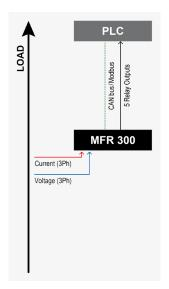
In this general application the device is used as a transducer with monitoring functions. The control does not operate any breaker.
