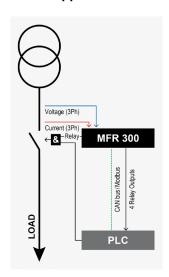
In this mains related application the device is used as a transducer with monitoring functions. The control can be used to open a breaker.
