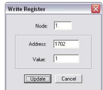
Figure 9-13: Modbus - write register - resetting the default values
