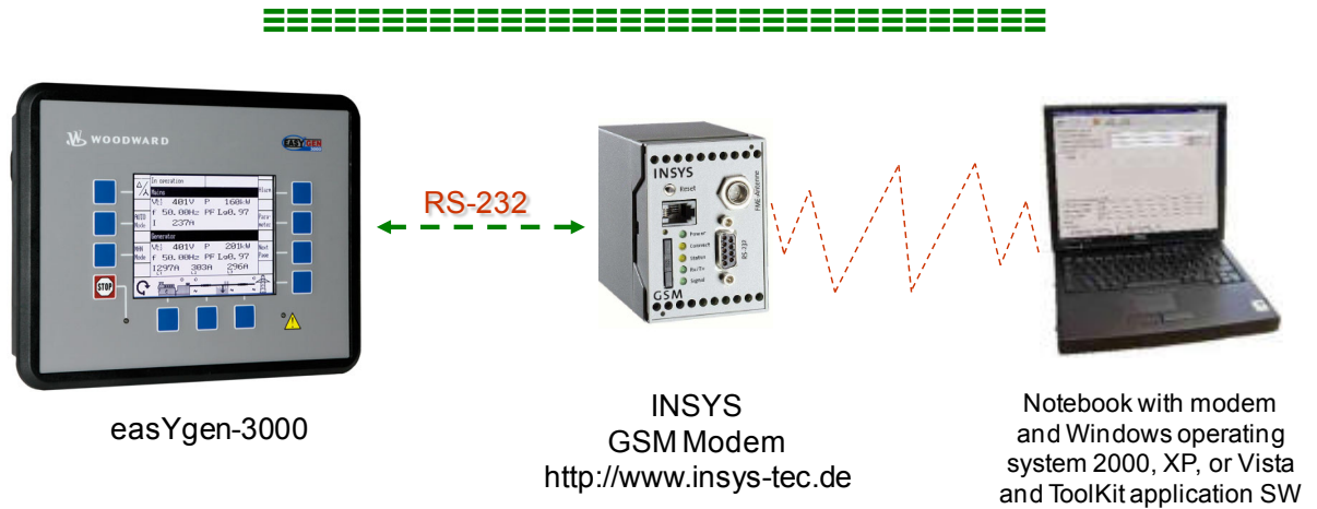
Figure 4-28: Connecting a GSM modem
