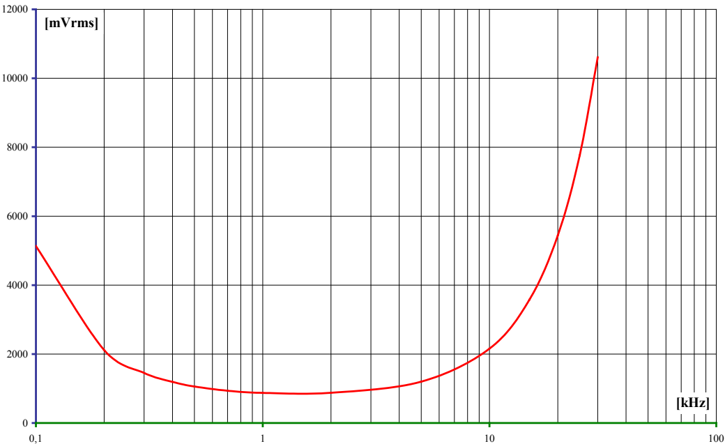
Figure 6-40: Minimal necessary input voltage depending on frequency
