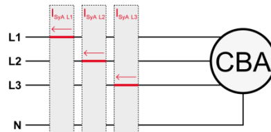
Figure 2-32: Current measuring – system A, L1 L2 L3
