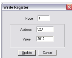
Fig. 368: Write register - acknowledge alarm message
