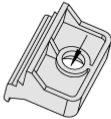
Fig. 12: Insert screws in clamps
