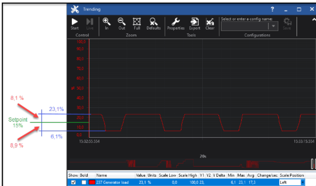
Fig. 204: The ToolKit trend shows the oscillating of a load step. The example shows that the dead band must be minimum 8.9\% + 1\% = 9.9\% that the oscillating is prevented.
