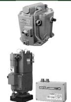
The **TG-13E** and **TG-17E** actuators are drop-in replacements for TG mechanical governors, and are self-contained electro-hydraulic actuators for use on steam turbines where isochronous control, load sharing, or other functions are required. They can be used with all available Woodward electronic governor controls and accessories.
