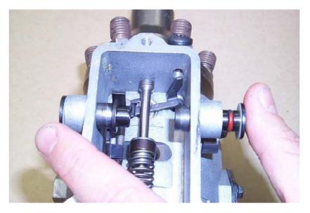
5. Install the new cover gasket into the groove on the L-Series (8404-5003). Install the L-Series assembly, with the linkage oriented as shown in the following photo. Do not force the cover into place—if the linkage is properly aligned, it will fit without being forced. The fork should engage the pump linkage. Tighten the three cover screws, torque to 4.0–5.1 N·m (35–45 lb-in).
