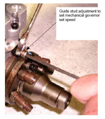
This completes the mechanical installation. Now the electrical harness will need to be installed on the engine.
