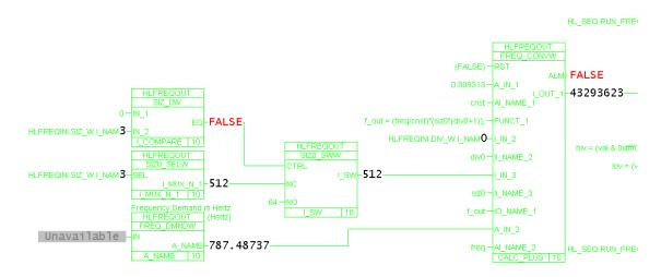
The above section of the GAP uses the function of  $(freq/cnst)^*(siz0^*(div0+1))$  to calculate the value required for the Highland card generate the requested frequency. Every count of the register used for the frequency is equal to 0.009 313 Hz. The number of points loaded into the wave memory is equal to the block size setup for the channel or  $(siz0^*(div0+1))$ .
