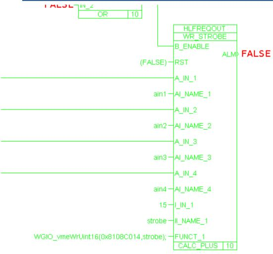
Block HLFREQOUT.WR\_STROBE writes the strobe bits for channels W, X, Y, and Z to Address C014. The strobes for each channel are bit addressed in this register i.e. channel Y = bit 2 (4hex). The code is set to strobe all four channels.
