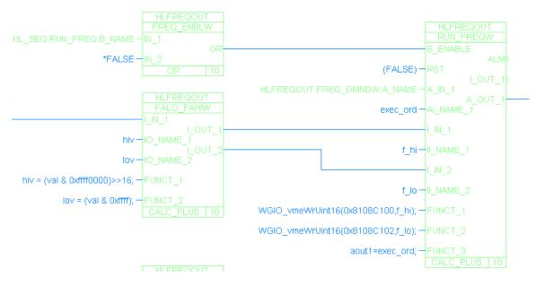
The calculated value needs to be written to two 16 bit registers located at address C100 and C102. Address C100 (f\_hi) is the MSB and C102 (f\_lo) is the LSB of the requested frequency value. Block HLFREQOUT.FALO\_FAHIW takes the 32bit value from I\_IN\_1 and splits it into 2 16 bit words to write to the addresses on the Highland card. Note that both of these addresses must be written anytime that the frequency is to be changed, and must be done with the strobe bit for the channel set to 0.
