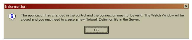
The new software is now loaded in the control. The EGCP-3 should go through a re-boot phase and after about 60 seconds, the screen should show valid data. The software can be verified by going to the password screen of the EGCP-3. On the bottom line of this display the software version is displayed. The software should now be 5418144K.
