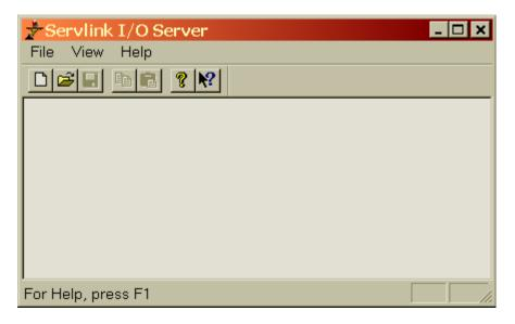
The first action to take inside the ServLink screen is to set up a new network definition file. Click once on  $\underline{\mathbf{F}}$ ile, and then on  $\underline{\mathbf{N}}$ ew as shown. The new network definition window will pop up on the computer screen.
