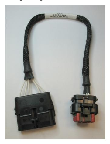
Figure 2-1. Example of a Flo-Tech to F-Series Adaptor Cable
