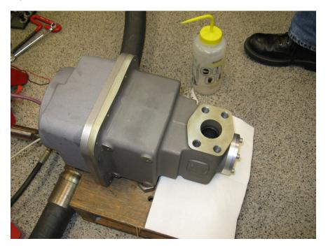
The valve should be actuated using a slow ramp triangle wave from either the Falcon Monitor (internal service tool) or from the Control System. The valve should be actuated from 0 to 100% valve position using a 0.05 Hz ramp.
