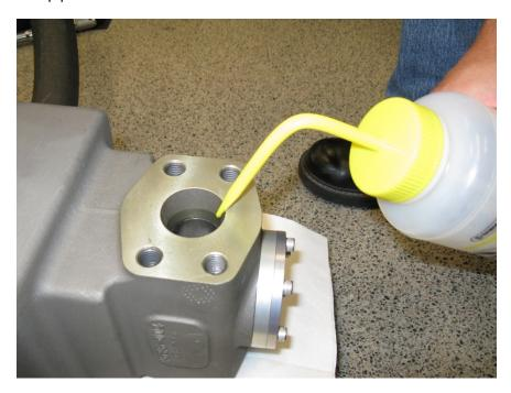
4. After the metering element and shoe are thoroughly cleaned, the area should be dried using low-pressure nitrogen or compressed air. Take care not to introduce impurities or oil.
