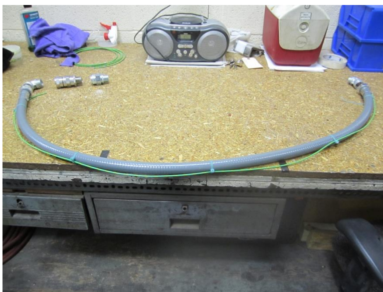
Figure 3-2. Tefzel Grounding Wiring Installation
