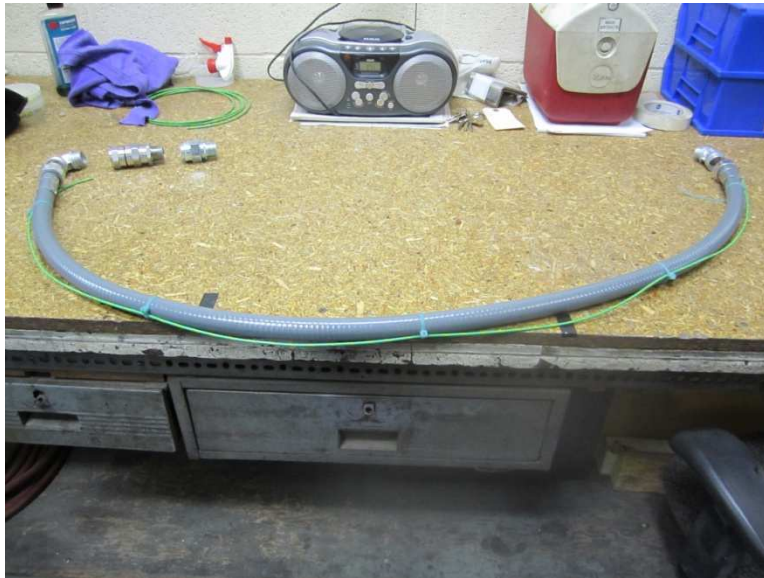
Figure 3-3. Tefzel Grounding Wiring Installation
