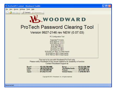
Connect to module A through the RS-232 Service Port on the ProTech and press the "Connect" button on the tool. The following screen will appear.
