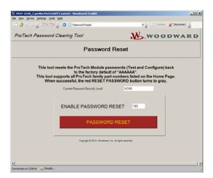
The Current Password Security Level should read NONE, indicating that the ProTech is not in Configuration mode. This is the correct reading for resetting the ProTech passwords.
